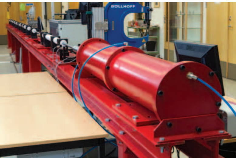
Figure 13 – Split-Hopkinson pressure bar. Photo: Ole Morten Melgård
