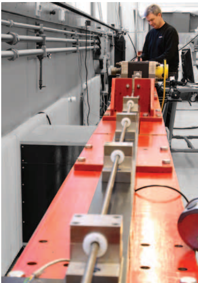
Figure 12 – Split-Hopkinson tension bar. Photo: Melinda Gaal
