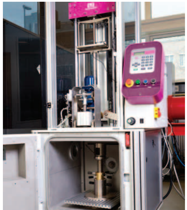
Figure 20 – Droptower impact system. Photo: Ole Morten Melgård
