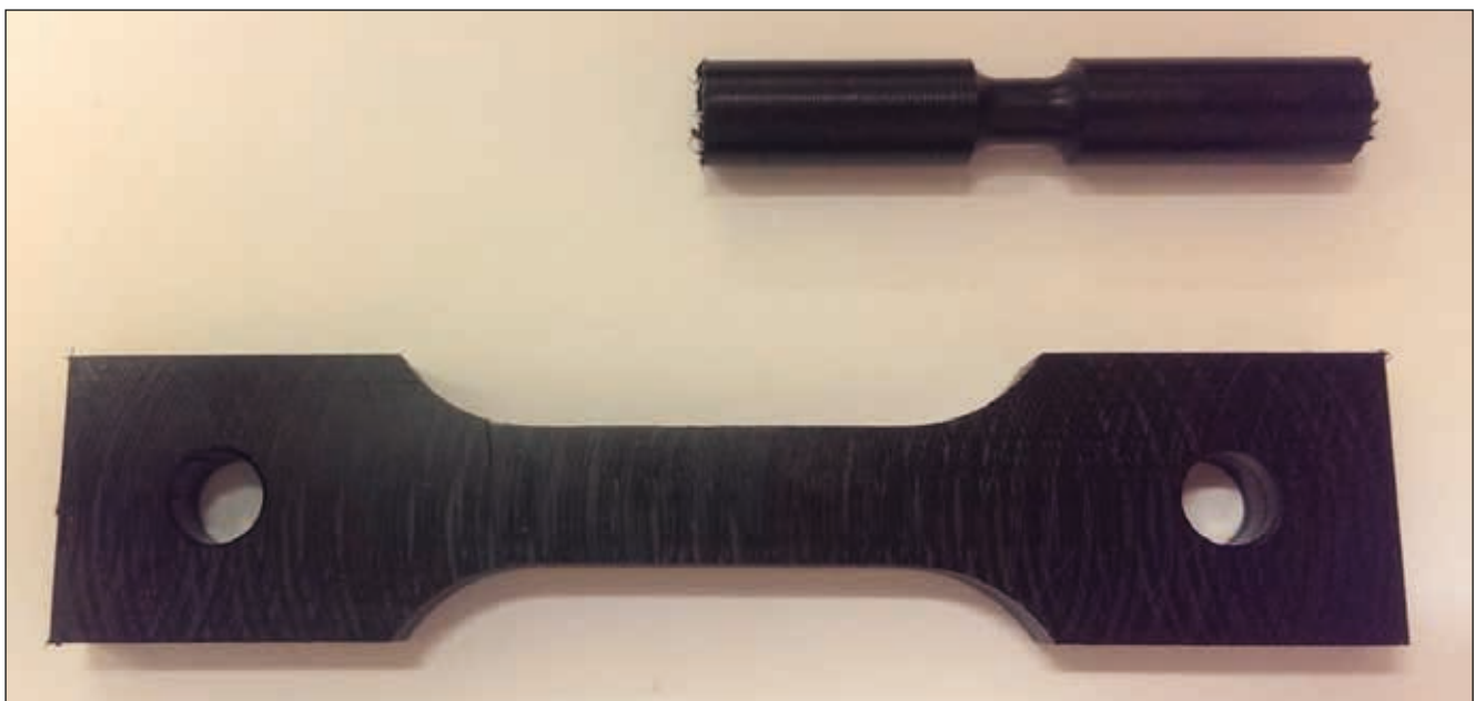
Figure 3 Improved tension test sample (circular cross-section) and conventional sample (rectangular cross-section).
