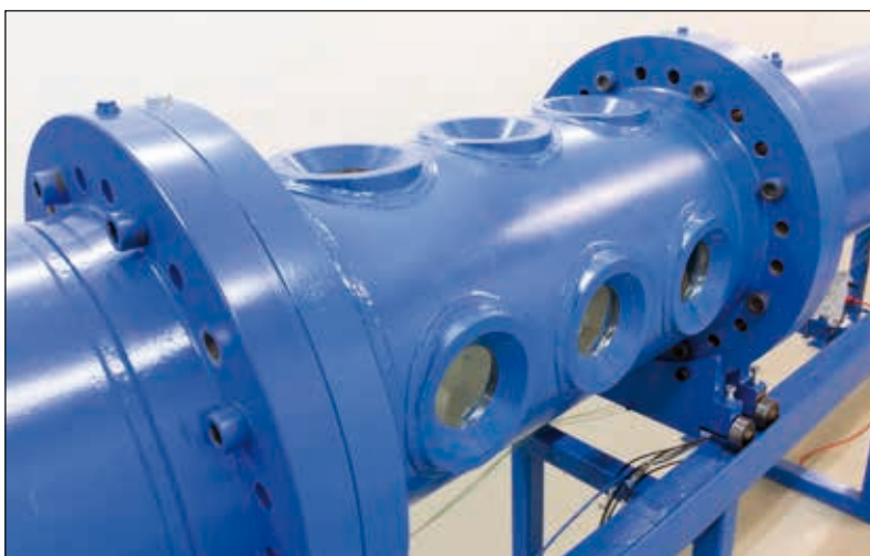
Figure 23 The window section.
