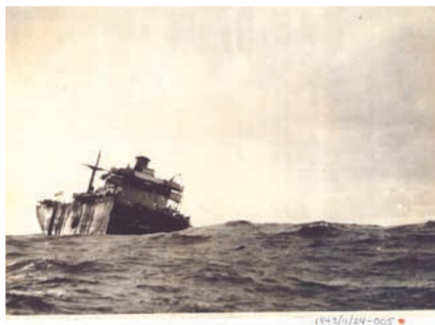
Liberty ship SS John P. Gaines broke in two and sank in a storm off the Alaskan coast on 24 November 1943. The steel became too brittle in the cold.
