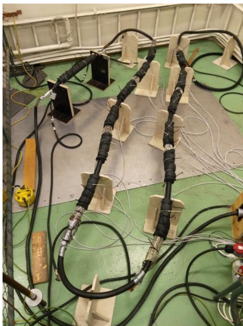
Figure 1: Picture of the test setup in the laboratory. The ground screen connections of type I to the left, type II to the right. Each ground screen connection is located underneath the black thermal insulation.
