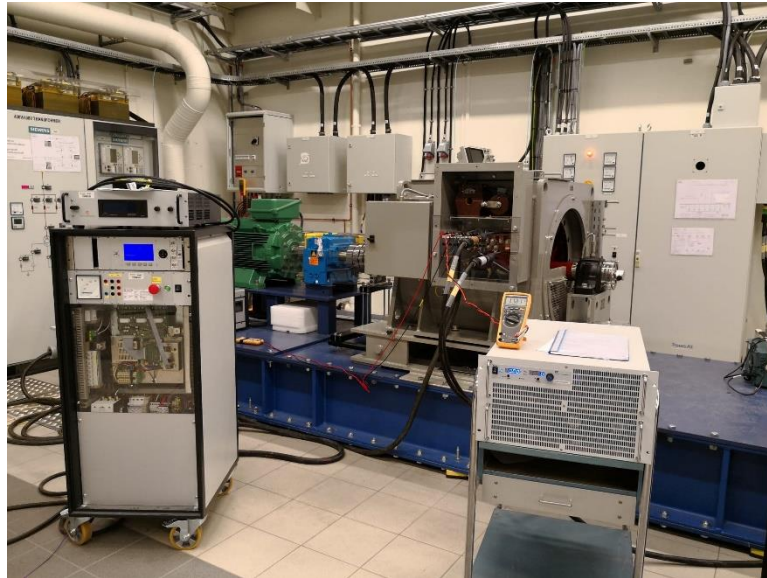
Experimental set-up of synchronous generator for fault detection purpose
