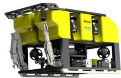
Fig. 1 – Argus Worker WROV rated at 175 hp ( \approx 130 kVA).
