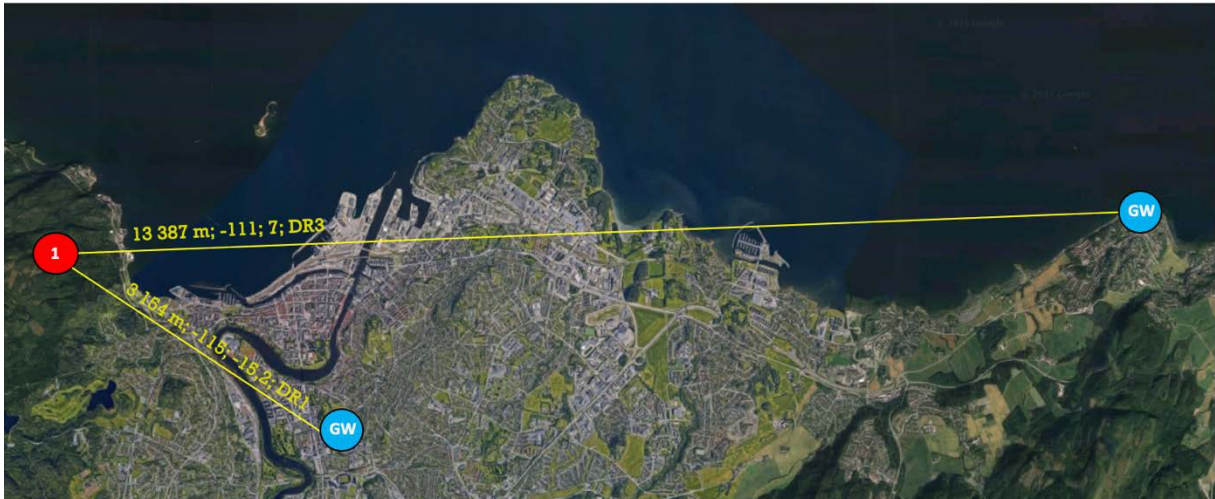
Signal qualities for GW connections from location 1 (Distance; RSSI; SNR; Data Rate)
