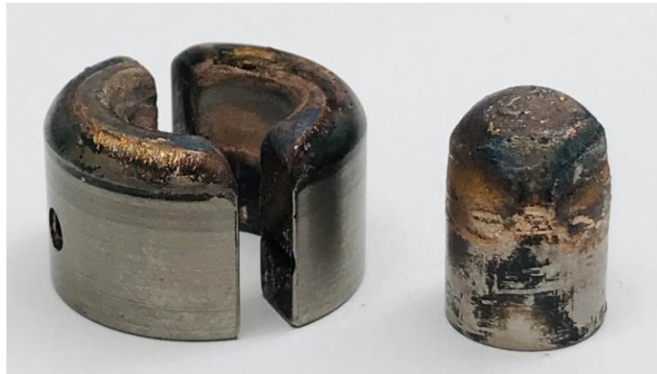
Eroded surface of arcing contacts after making operation.
