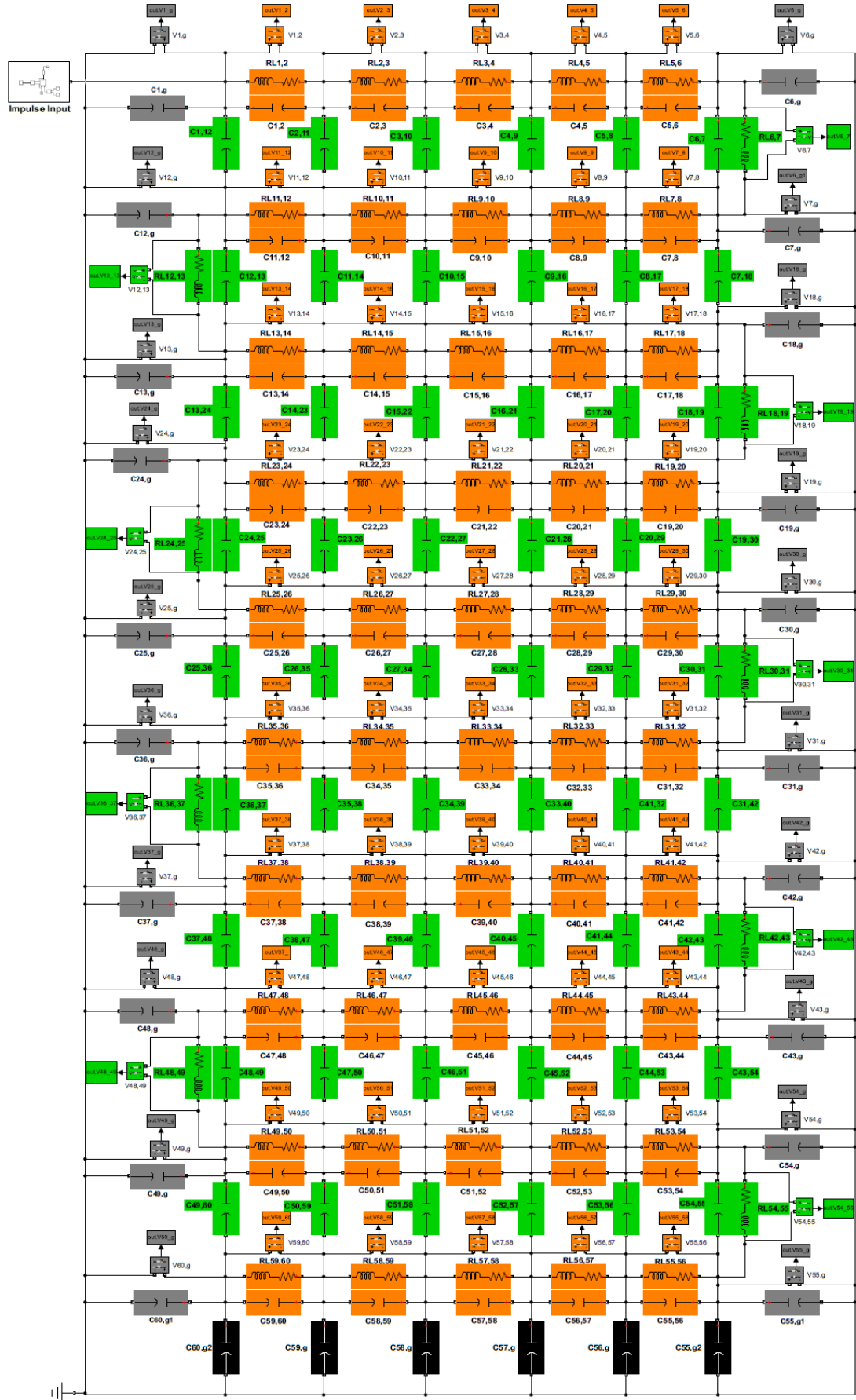
Figure 3: Implementation of LP model for single slot winding in MATLAB/Simulink.
