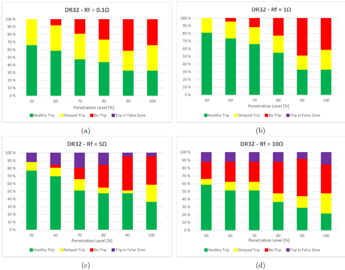
Figure 2: Impact of fault resistance on DR32, including simulations for unsymmetrical faults only, all control strategies, and divided between all penetration levels. a) R_f = 0.1\Omega , b) R_f = 1\Omega , c) R_f = 5\Omega and d) R_f = 10\Omega .
