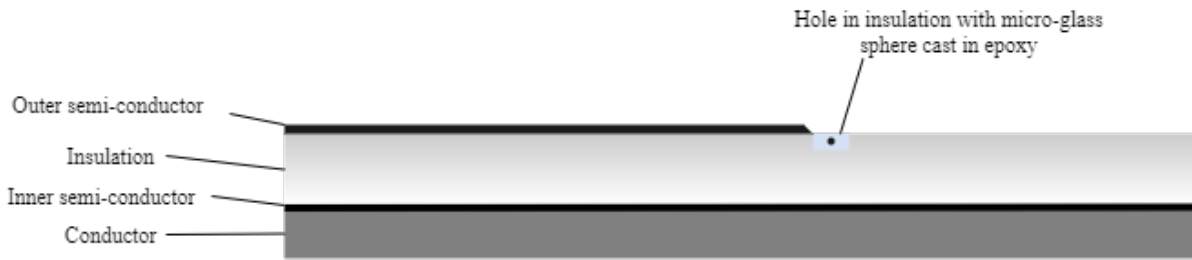
Figur 2 Micro-glass sphere implementation in cable insulation with the use of epoxy
