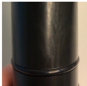
Figure 2: Image of rubber gasket placed in the milled slot.
