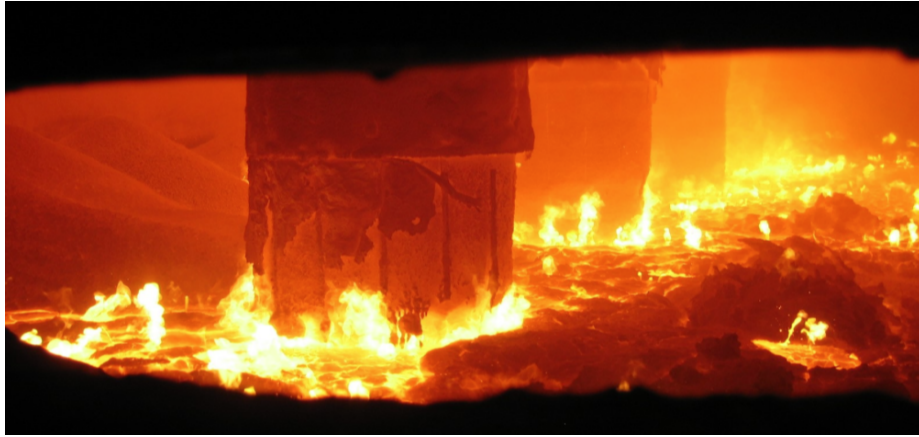
Figure 4.1: Søderberg electrodes at work in a smelting furnace. Photo courtesy of the main webpage https://www.elkem.com/carbon/about-elkem-carbon/
