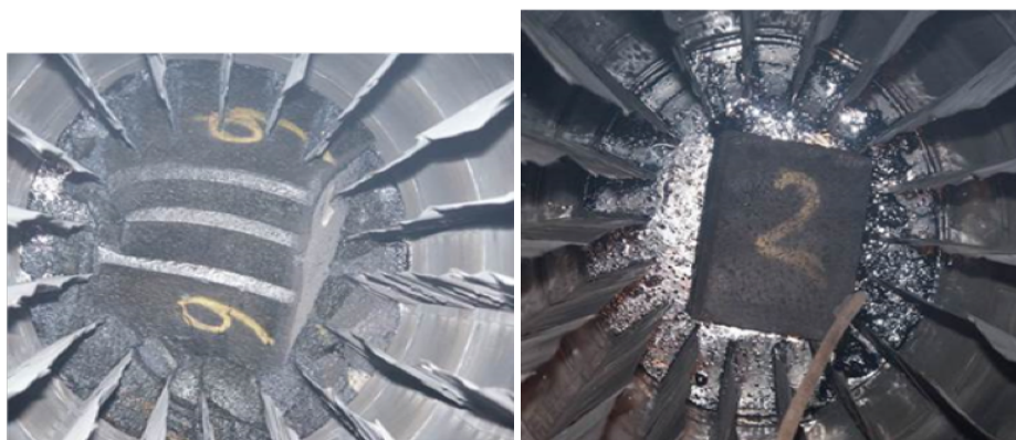
Figure 4.4: Photos taken looking directly down on Söderberg electrodes, illustrating the difference between a properly operating electrode (left, number 6), and an electrode affected by segregation (right, number 2). The fins inside the steel tube provide extra grip for the moving electrode near the bottom. Number 2 has a square block fed in at the top rather than a cylinder. Number 6 has multiple slabs fed in at the top, which are partially slumped.
