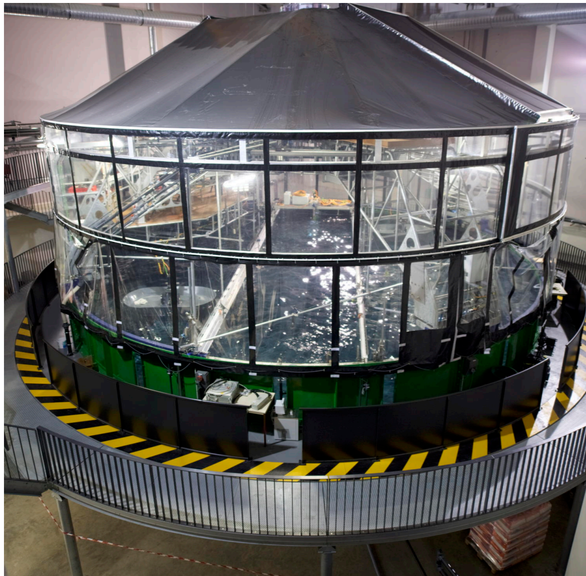
13m diameter, 100 tons of water, 2 tons of salt, rotation up to 2 rpm
