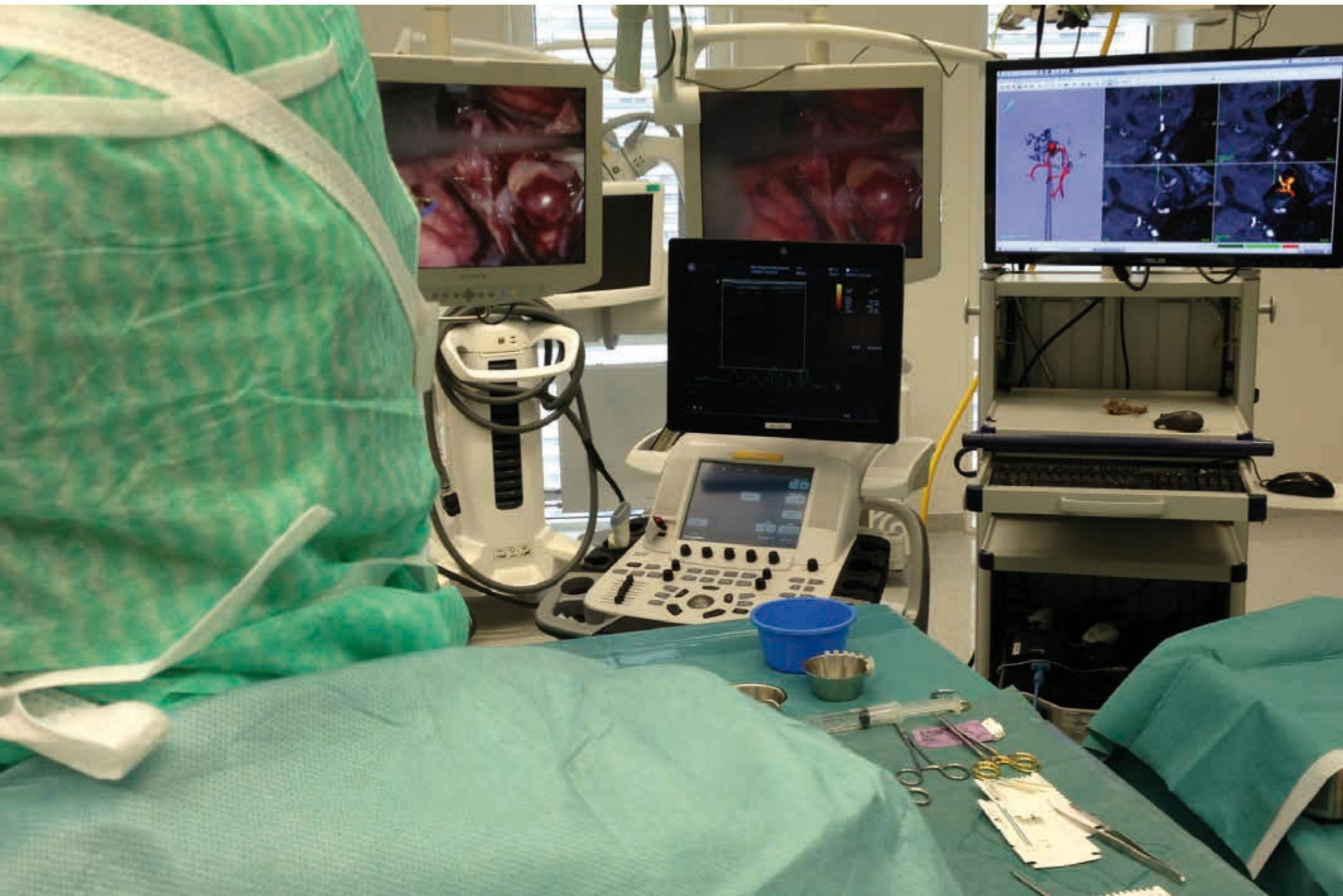
With the new system, ultrasound is used to continuously update the pre-surgery MR images during surgery.
