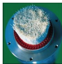
Bundle of hollow fibre membranes in an industrial module—packing densities can be up to 30 000 m 2 /m 3
