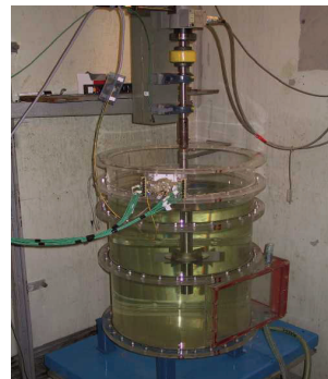
A stirred tank used for studies of heat transfer and flow phenomena.
