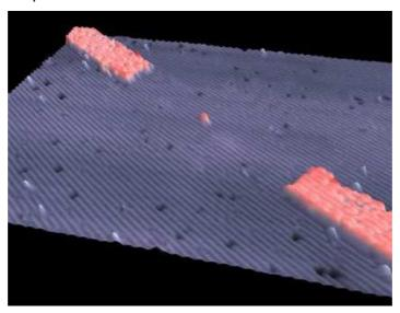
A (single-electron) transistor (in red) made by accurately positioning a single P atom (red spot in the middle) on the surface of a silicon crystal (blue), with a scanning tunnelling microscope (STM) tip [4].
