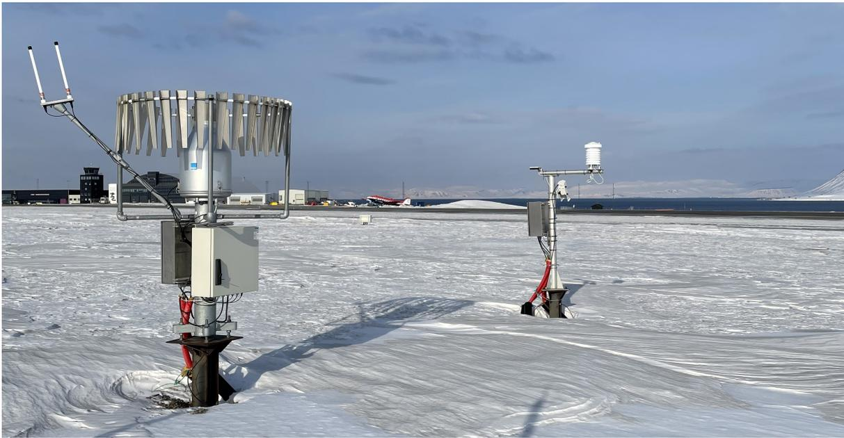
*Figure 17: Photo of parts of the weather station at the airport. Precipitation gauge on the left, temperature/humidity sensor and snow depth sensor on the right.*
