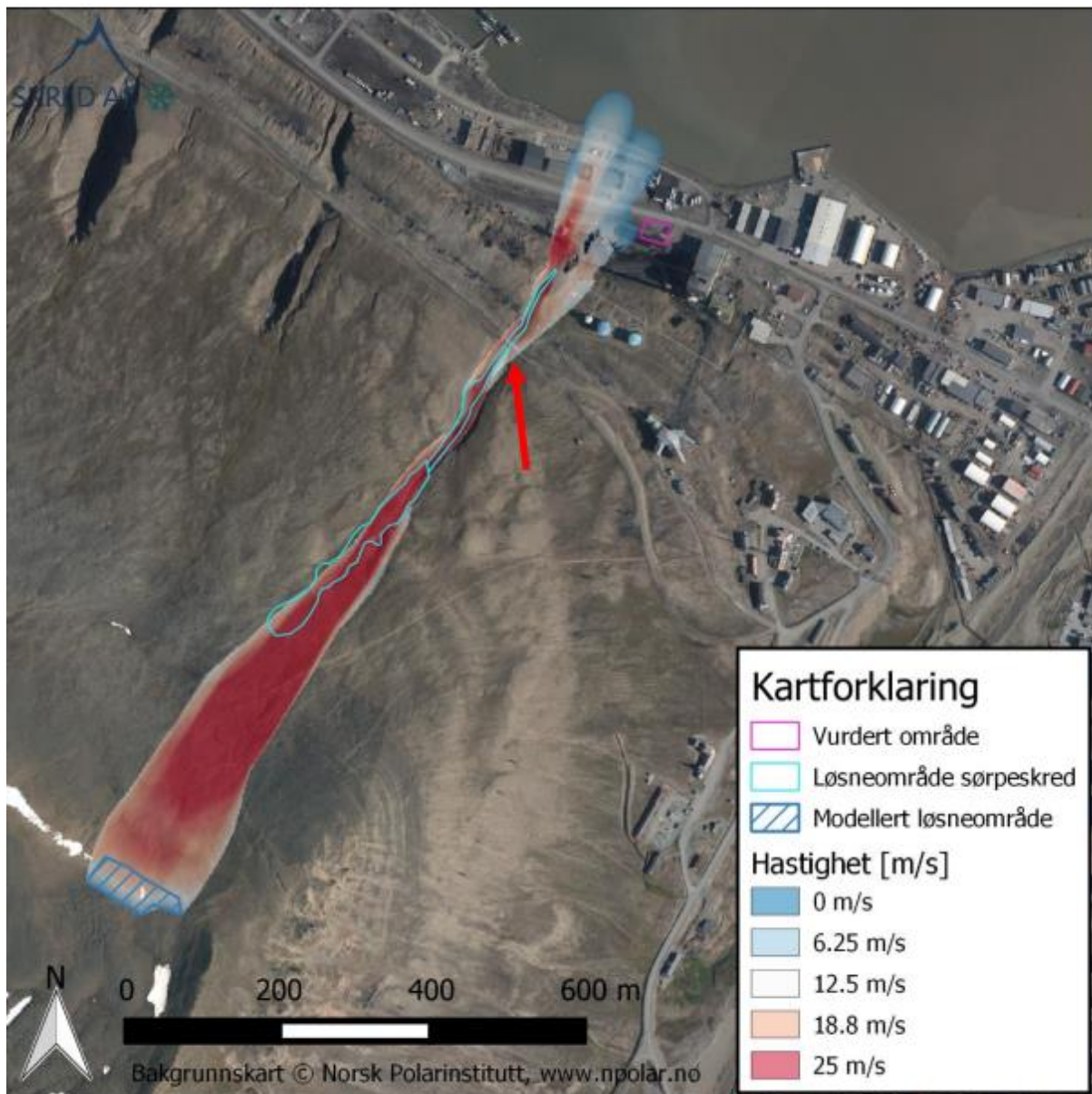
Figure 16. Debris flow hazard map of Longyearbyen power plant (NVE, 2016)
