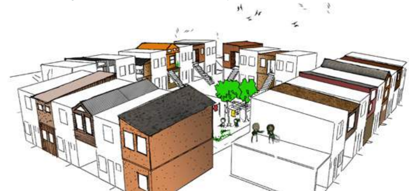
Fig.31 - Sketch showing cluster around common courtyard with possible increments
