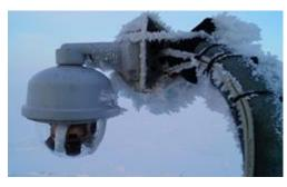
3 camera systems with 11 lenses for optical ice condition and environmental monitoring (Martin Heyn)
