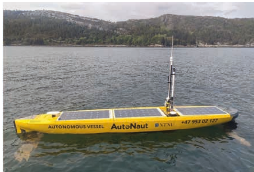
Figure 7: The AutoNaut: a wave-propelled surface vehicle.
