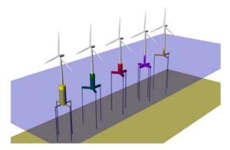
Figure 47: Tension leg platform wind turbines (TLPWTs).
