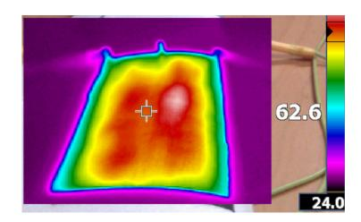
Figure 14: Thermal image of the effect of heating on the leading edge of a UAV wing section with carbon nanotube coating.
