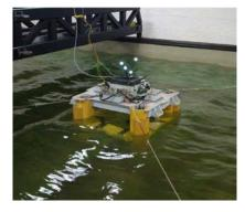
**Figure 59:** CyberRig I moored and positioned in waves.
