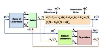
Figure 26: Supervisory control architecture.
