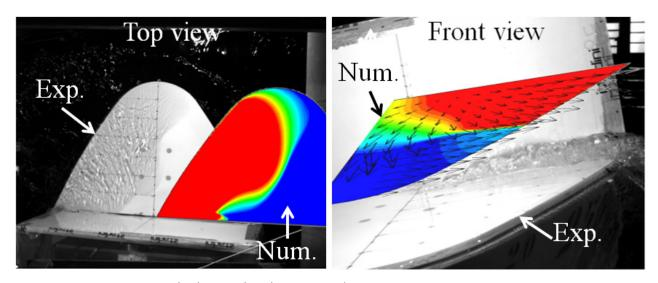
**Figure 20:** Phases of water on (left) and off (right) deck for  $\omega_{4n0}/\omega=0.402$  and kA=0.25. For the numerics: the contour levels indicate the water height and the vectors indicate the water speed.
