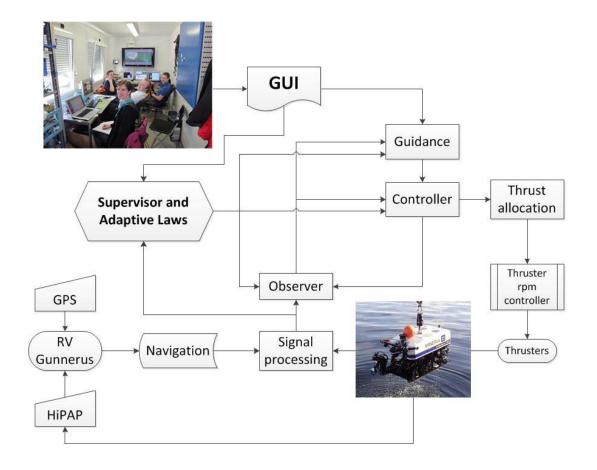
Figure 9: ROV motion control architecture.
