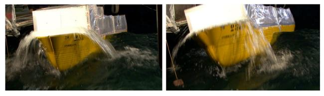
Figure 22: Run 44 (left) and run 46 (right) at the time instant as a wave crest at mid-ship.
