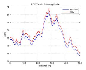
Figure 11: Research campaign Tautra: ROV depth trace and the estimated terrain profile from DVL measurements.
