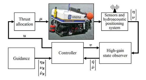
**Figure 41:** Block diagram of the output feedback control system. The block corresponding to the controlled plant is illustrated here by the NTNU's ROV Minerva.
