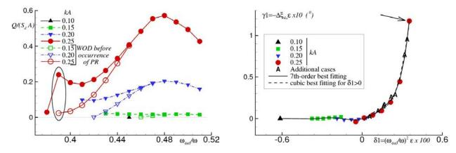
**Figure 21:** Maximum volume of shipped water Q in steady-state conditions before and after PR.  $S_d$  is the deck area. Right: Scaling law for the variation of the steady-state roll amplitude  $\mathbf{D}\zeta_d$  caused by WOD loads.
