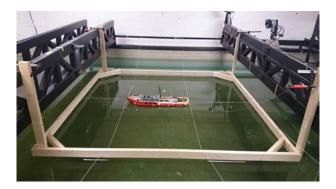
**Figure 62:** Hydrodynamic parameter identification for C/S Enterprise I.
