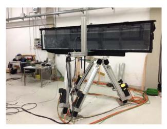
**Figure 69:** Setup for 2D tests on water-oil-boom interactions.
