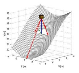
Figure 10: DVL beams (red) and linear sea floor (white) approximation using 3 of 4 beams in addition to estimation of altitude (blue) and gradient vector (green).
