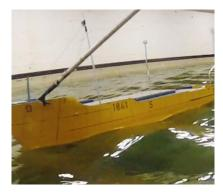
**Figure 61:** CyberShip III used in DP testing.
