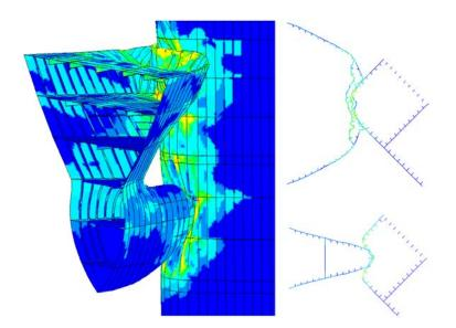
Figure 30: Simulation of penetration and damage distribution in bow-platform column impact.
