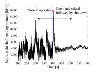
**Figure 45:** Time series of the main-shaft bending moment in grid loss and blade seize followed by shutdown; landbased turbine; mean wind speed=17 m/s; turbulence intensity=0.2; time of fault occurrence=400 s; pitch rate=8 deg/s; HAWC2 simulation.
