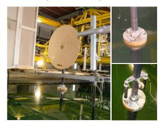
**Figure 49:** The STC test model at INSEAN (right-top: MWL survival mode with the torus fixed to the spar at mean water level; right-bottom: operational mode with the torus connected to the spar by two pneumatic cylinders to model the PTO damping).
