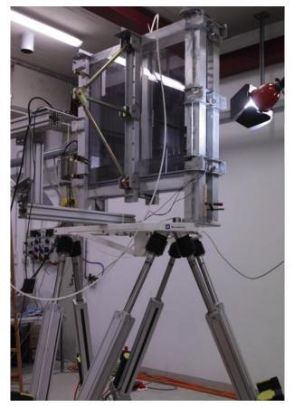
**Figure 68:** Setup for 2D sloshing tests on a tank with a deformable plate on the left side wall.
