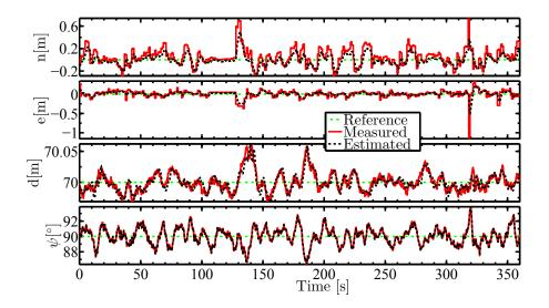
Figure 43: DP test: Position and heading angle in the NED frame.
