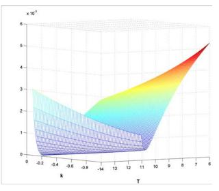
**Figure 27:** Distance of the Nomoto systems with different k and T values from the Nomoto system with k = -0.15 and T = 8 as a function of k and T.
