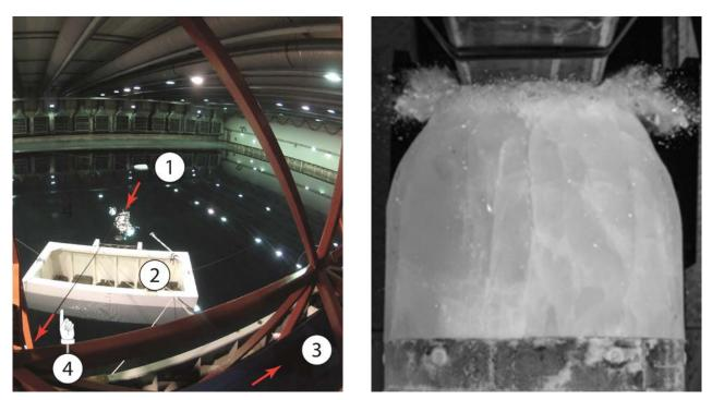
Figure 32: a) Towing impact test, b) High-speed impact experiment.
