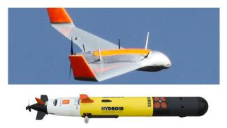
**Figure 6a-b:** The figure shows the X8 UAV equipped with five antennas to support the different radio communication needs of AUV Remus 100's Wi-Fi link, ground station link, and telemetry.
