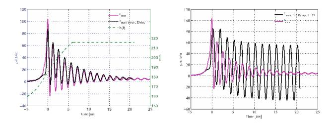
**Figure 24:** Left: Hybrid model (black line) and experimental (magenta line) time histories of the strain at the centre of the beam. Dashed line represents the instantaneous variation of the wetted part of the wall. Right: Simplified model (black line) and experimental (magenta line) time histories of the strains at the centre of the beam.
