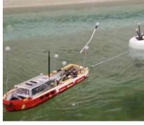
**Figure 60:** C/S Enterprise I set up as an iceberg towing vessel.
