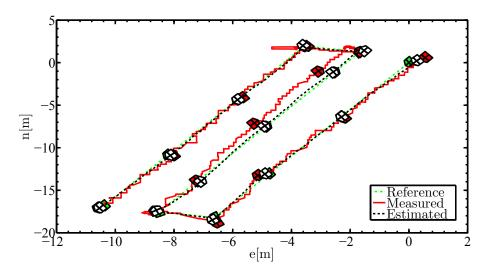
Figure 42: Trajectory tracking test: Top view of the North-East plane.
