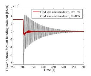
**Figure 46:** Effect of pitch rate on the tower-bottom bending moment during shutdown; constant wind speed=20 m/s; land-based wind turbine; Simo-Riflex-AeroDyn simulation, *Pr=pitch rate.*
