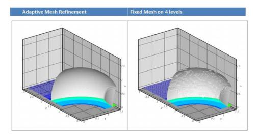
**Figure 28:** Adaptive mesh versus fixed discretisation: snapshot of the surface with maximum pressure at the time of wave reflection from a wall.
