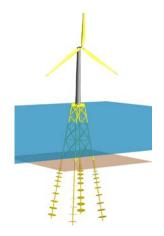
**Figure 3**: Model of jacket-supported wind turbine with pile-soil modelling.
