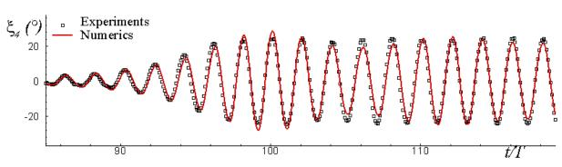
Figure 19: Parametric roll for  $\omega_{4n0}/\omega$  =0.402 and kA=0.25.
