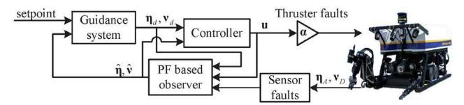
Figure 8: Fault-tolerant control system of underwater robot.
