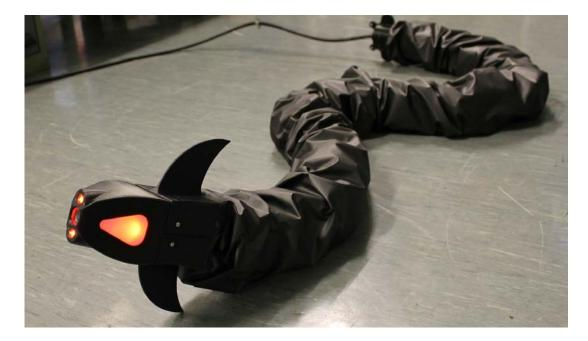
Figure 44: The snake robot Mamba in the NTNU Snake Robotics Laboratory.
