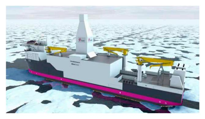
Figure 61: The Inocean design of Statoil Cat I Arctic drilling unit. Illustration: Inocean.
