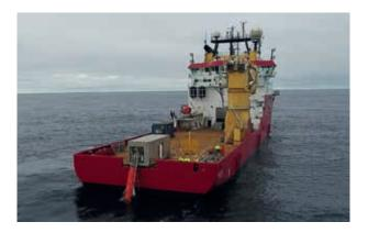
*Figure 58:* AUV Hugin HUS on the stinger during recovery on OCV Polar King after a successful dive to 3000 m on the AMOR.
