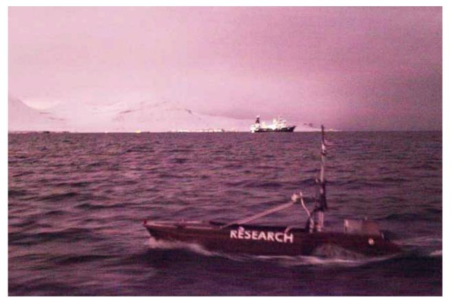
*Figure 59:* USV Jetyak in the Polar Night measuring light spectra and acoustic reflections to investigate the vertical migration of zooplankton.
