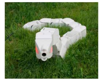
*Figure 20*: Mamba – a novel snake robot prototype with force/ torque sensors for sensing obstacles in the environment.
