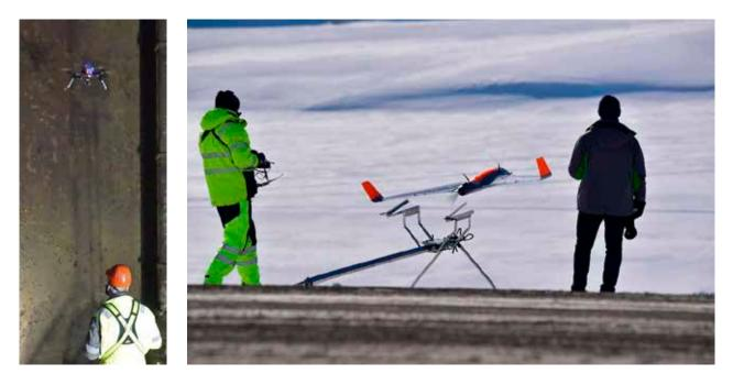
*Figure 55 (left):* NTNU AMOS testing UAV technology for inspection of a tank in Njord B with Statoil. Photo: Kristian Klausen, NTNU. *Figure 56:* The launch of NTNU's X8 UAV from Ny-Ålesund, Svalbard. Photo: Kjell Sture Johansen, NORUT Tromsø.
