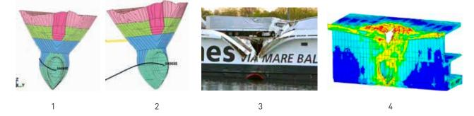
**Figure 45:** Panels 1 and 2: collision of a ship with a semis-submersible column. 1: early stage with rolling and yawing away from platform. 2: later stage with rolling back and hitting the platform. The yellow beam in the rear represents the hull girder motion. Panels 3 and 4: collision between the Ropax vessel URD and the ferry Nils Holgerson. 3: actual damage. 4: simulated damage to ship side.
