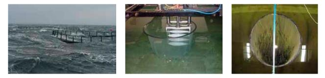
*Figure 7:* Left: overtopping and out-of-water event for the floater of a fish farm without a net in a storm (photo: Marius Dahle Olsen). Centre and right: experiments on a net cage with 9 artificial fish (centre) and with 814 real fish (right) in regular waves and current.
