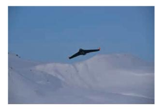
Figure 30: X8 Skywalker, fitted with the NTNU AMOS IPS, flying over Kongsfjorden, Ny-Ålesund, Svalbard.
