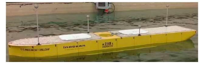
Figure 62: The model ship C/S Inocean Cat I Drillship in MC-Lab. Photo: Jon Bjørnø, NTNU.
