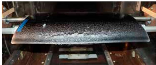
**Figure 5:** The upper and lower part show different kinds of icing accretion test during severe icing conditions.
