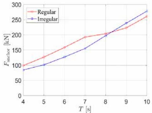
**Figure 2:** Left: Numerical net-based fish farm in regular waves (period  $T = 6$ , height  $H = 2.5$  m), without current (top) and with current speed  $U_\infty = 0.5$  m/s (bottom). Right: Comparison of the maximum anchor loads by numerical calculations in irregular waves and equivalent regular waves. The considered regular wave steepness is  $H\lambda = 1/15$ , the current velocity is  $U_\infty = 0.7$  m/s. The significant wave heights for irregular waves are given as  $H_s = H/1.9$ .
