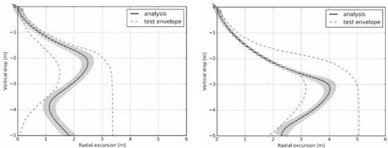
**Figure 5:** Numerical drop trajectory for a submerged drop and corresponding envelope from Aanesland's tests. Left: drop angle = 30°. Right: drop angle = 45° (right).
