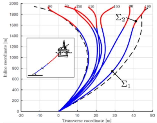
**Figure 10:** Snapshots at given times of a substructured mooring line, when subjected to an exogenous load. The numerical substructure is represented in blue and the physical substructure in red.
