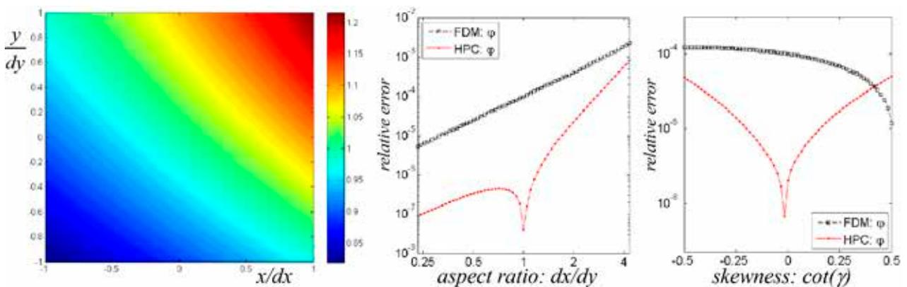
**Figure 6:** Local analysis for a cell with dimensions  $dx$ ,  $dy$ , assuming a true velocity potential  $\phi$  with contour plot in the left. Relative error as a function of cell aspect ratio  $dx/dy$  (middle) and of cell skewness  $\cot \gamma$  (right) for a standard finite-difference method (FDM) with local 4th-order accuracy and for HPC. The latter allows local 8th-order accuracy.
