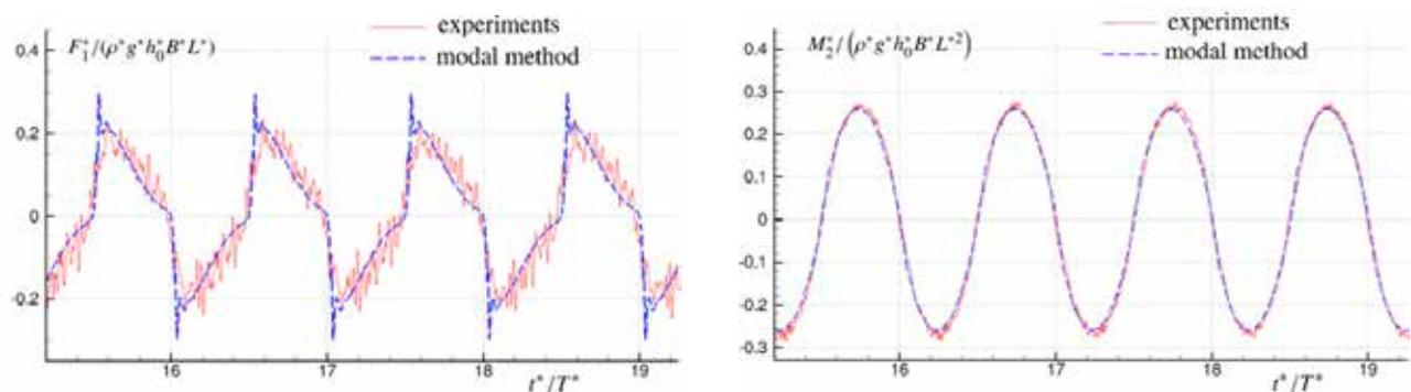
**Figure 4:** Evolution of global force (left) and moment (right) for  $\theta_0 = 4^\circ$ ,  $\sigma/\sigma_r = 1.0027$ .  $\theta_0$  and  $\sigma=2\pi/T$  are roll excitation amplitude and frequency, respectively.  $\sigma_r$  is the first linear resonant frequency.  $L$ ,  $B$  and  $h_0$  are the tank length, the tank width and the filling depth, respectively. Variables with symbol \* are made non-dimensional.
