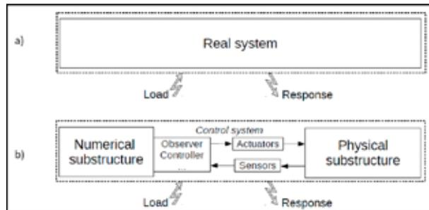
**Figure 9:** Partition of the system under study into a physical and a numerical substructure, connected through a control system. The fidelity of the cyber-physical empirical setup represented in b) quantifies how close its responses of interest are from those of a).
