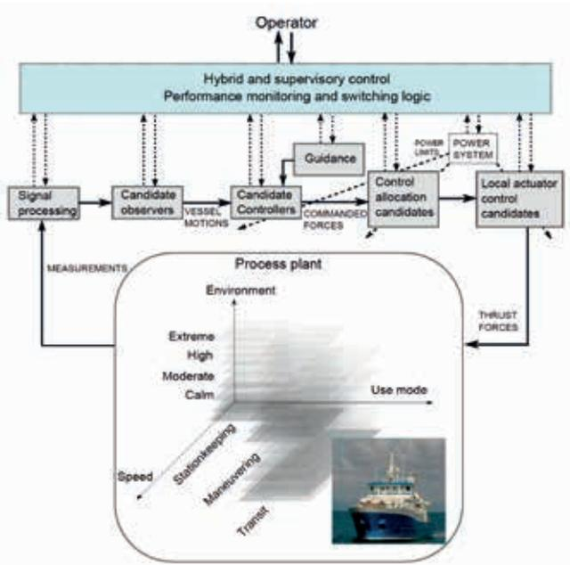
Figure 12: Block diagram of a hybrid control system for a marine vessel in an unknown environment.
