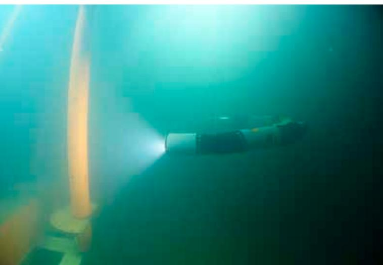
**Figure 1:** The Eelume articulated intervention-AUV inspecting a subsea installation (Courtesy: Eelume)
