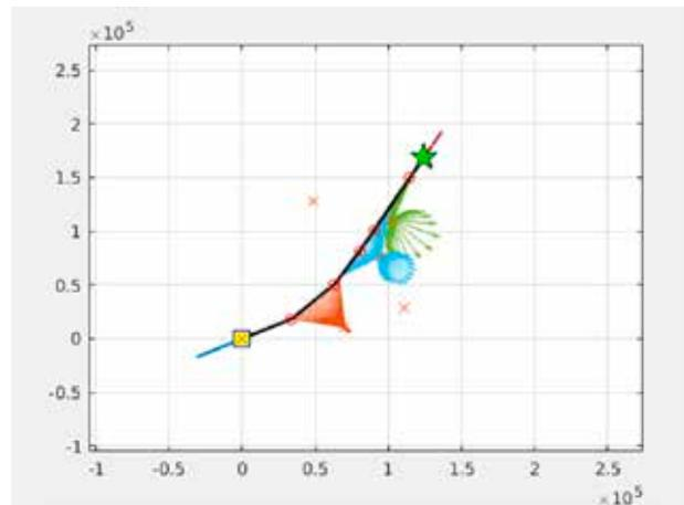
Figure 5: The optimal path from the starting location (yellow) to the final location (green). The red crosses mark possible emergency landing sites. It is indicated which emergency landing site should be chosen at each point along the optimal path.
