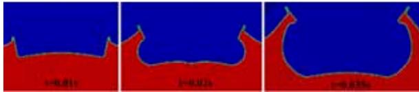
**Figure 17:** Snapshots of the plate deformation and flow field during water entry; initial impact velocity is 10 m/s
