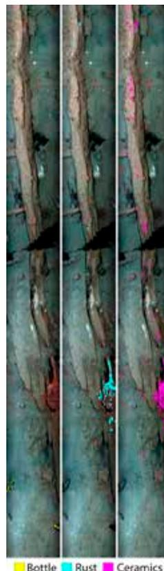
**Figure 5 (left):** Supervised SAM classifications of a UHI-based photomosaic of a wreck transect. From left: glass bottle, rust and ceramic.
