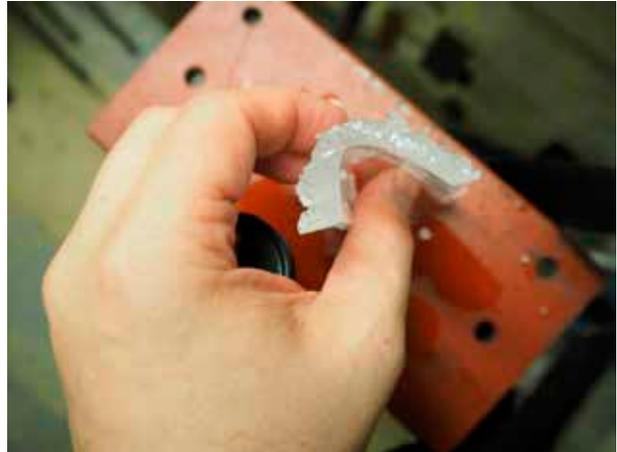
**Figure 4:** Examples of icing that was built up on the leading edge of wing during tests
