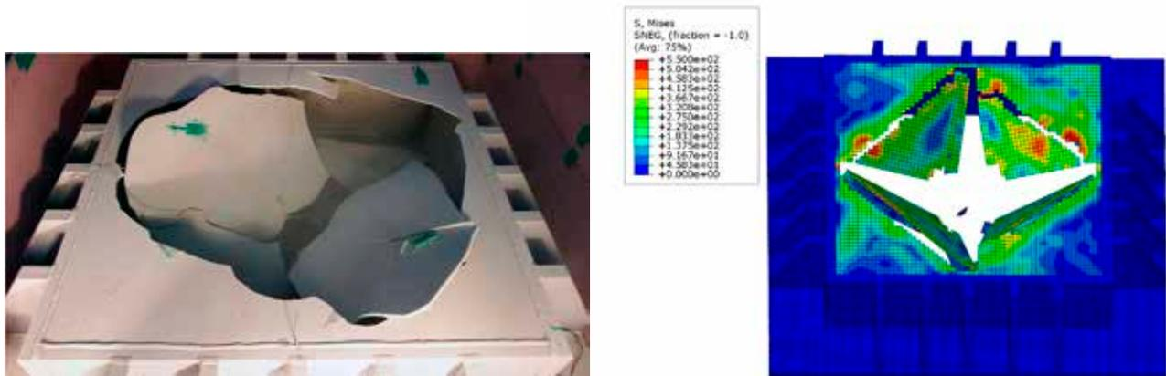
**Figure 14:** Left: Drop test carried at a temperature of  $-100^{\circ}\text{C}$ . (Kim KJ, Lee JH, Park DK, Jung BG, Han X, Paik JK. An experimental and numerical study on non-linear impact responses of steel-plated structures in an Arctic environment. *I.J of Impact Engineering*. 2016;93:99-115). Right Numerical prediction of the deformation mode. The fringe plot shows the von Mises stress field (in MPa) at the end of the simulation.
