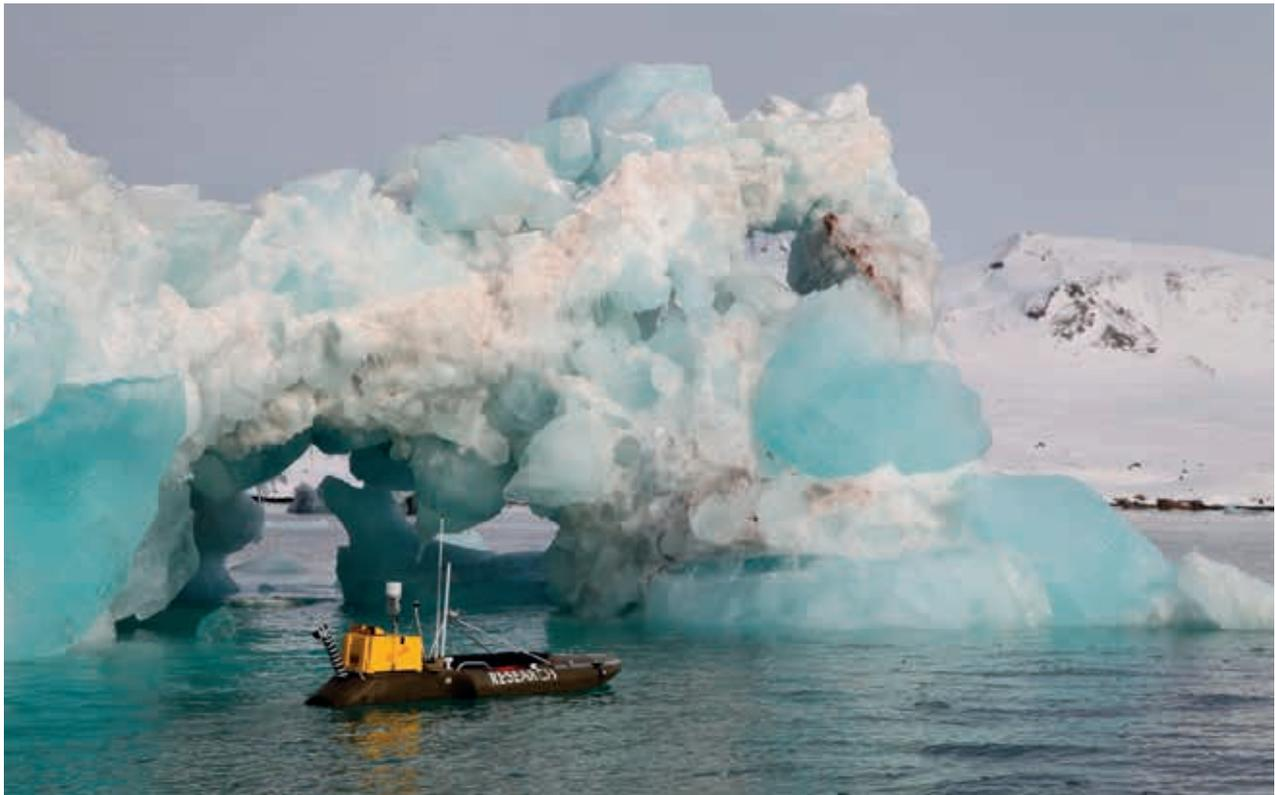
**Figure 1:** ASV Jetyak in Krossfjorden on Svalbard during a field campaign in April 2018
