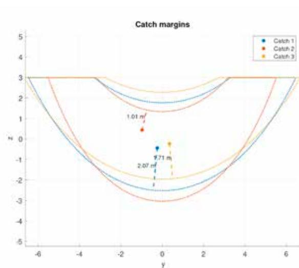
**Figure 3:** Margins for missing the catch for each of the three catches. The smallest margin and direction are marked.
