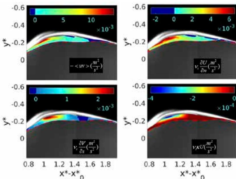
**Figure 8:** From left to right and from top to bottom: spatial maps at the stage (iii), of the Reynolds stress (top left), mean simple shear (top right), streamline curvature (bottom left) and geometric curvature (bottom right), respectively. The dashed red line gives the lower boundary of the turbulent region. Variables with the symbol \* are made non-dimensional.  $x^*_0$  indicates the origin of the image.
