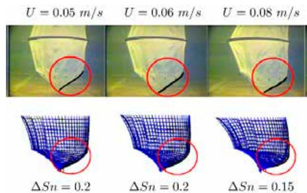
**Figure 3:** Fish farm in current. Left: Experimental relative drag change  $\Delta F_D/F_D$  caused by live fish. Right: Experimental (top) and numerical (bottom) net deformation in the experiment with 814 live fish. The area inside the red circle indicates the touching area.  $\Delta S_n$  represents the increase of solidity ratio at the back-cone part of the cage modeled in the calculations.
