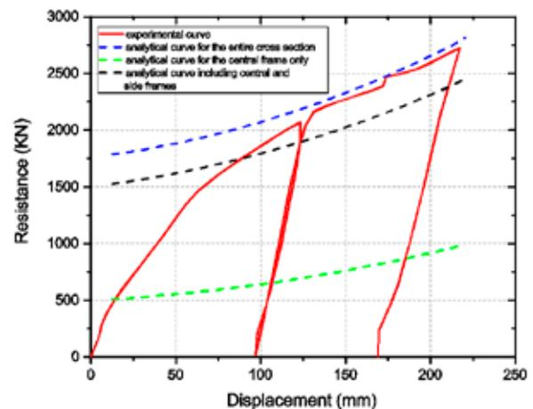
Figure 16 Left: Deformed full-scale ship grillage after loading with a cone shaped ice indenter. Right: Force –displacement curve from the experiments and prediction by the theoretical model.
