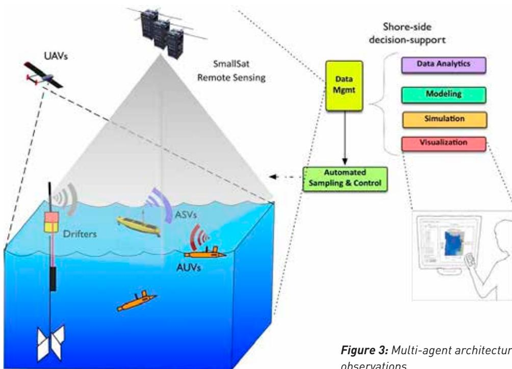
**Figure 3:** Multi-agent architecture for synoptic ocean observations
