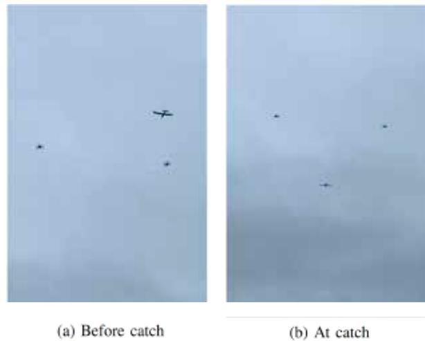
**Figure 2:** Pictures from the experiments at Eggemoen jointly with Maritime Robotics AS. Part (a) shows the moment just before the catch. Part (b) shows the moment of the catch. Notice that the hook from the catch line is attached to the multirotor line, but the fixed-wing UAV is still flying.
