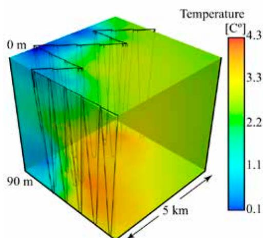
**Figure 3:** Path generated from measurements of the front. The cold water masses are shown as blue in the figure, and the black line illustrates the path of the robot.
