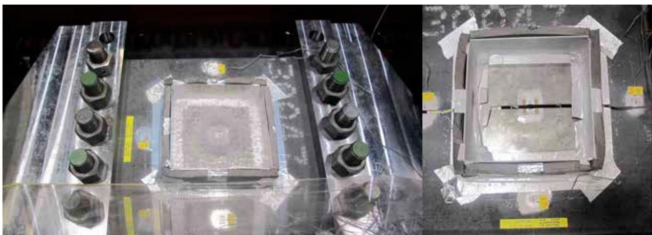
**Figure 15:** Left: Plate with initial crack in the middle subjected to cooling from liquid Nitrogen. Right: Brittle crack propagated from the middle crack and stopped close to plate edges with higher temperatures.
