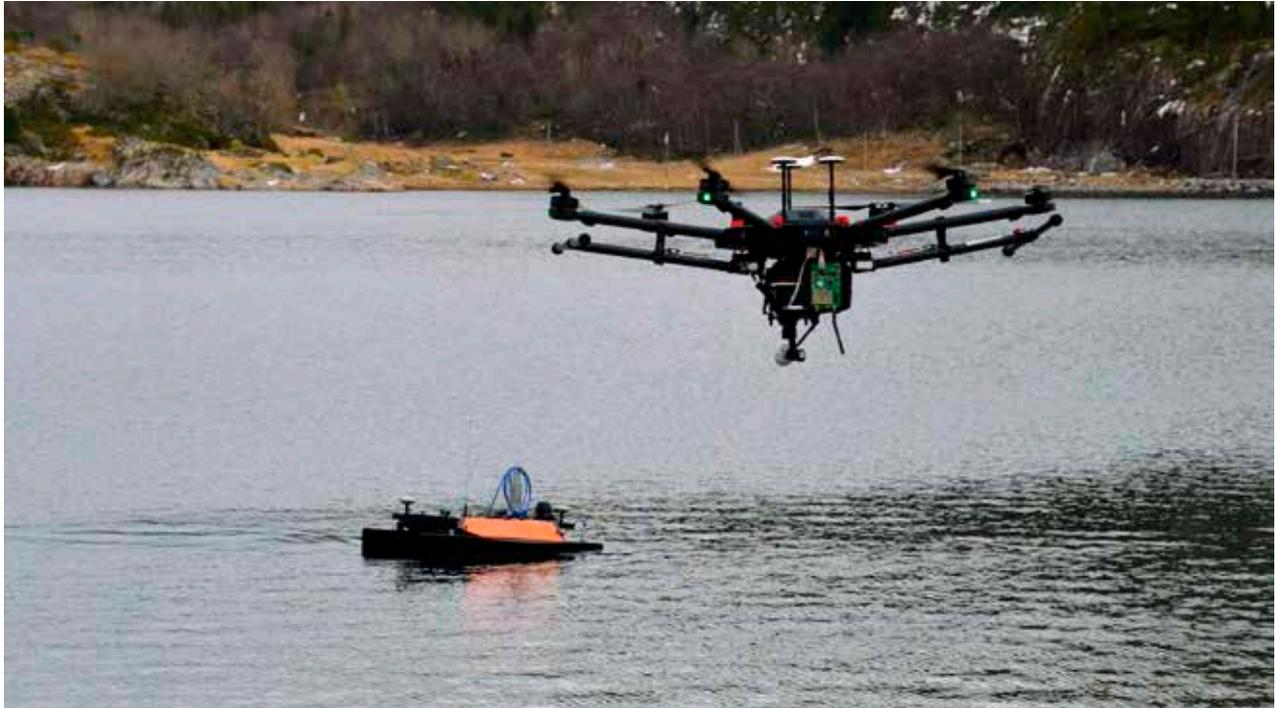
**Figure 9 (above):** Flying over, a hexacopter carrying a prototype hyperspectral instrument developed in partnership between UNIS and NTNU, references P1-R7 and P1-R9. On the water surface is a Maritime Robotics Otter USV equipped with an underwater hyperspectral imager (UHI) made by Ecotone. Both assets were operated by Maritime Robotics.
