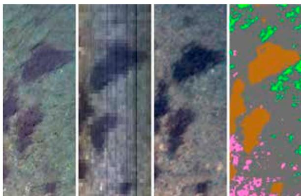
**Figure 11:** Airborne payload data. From left to right, first an image captured by the high resolution RGB camera, then an RGB representation of the hyperspectral data of the same region. On the third panel, an RGB representation of the same hyperspectral data after enhancement through fusion with the high resolution RGB image. Finally, classification using the same classes as in the UHI images.
