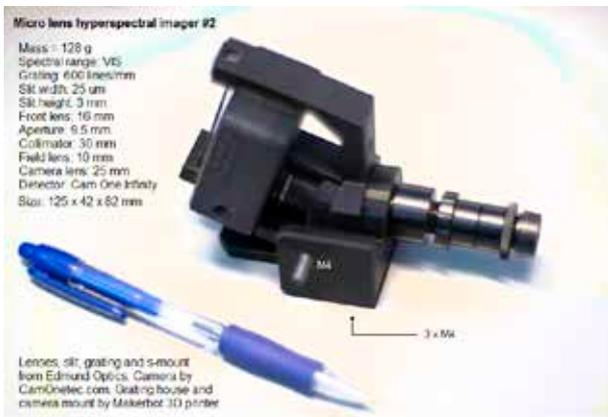
**Figure 6:** Second prototype of Hyper Spectral Imager (HSI) for drone operations
