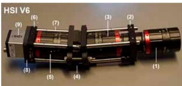
**Figure 7:** Assembled HSI V6 instrument using a standard USB 3.0 iDS camera head. (1) front lens, (2) CP12 cage plate, (3) collimator lens, (4) 3D printed grating holder, (5) camera lens, (6) CP03/M cage plate, (7) steel rods, (8) 3D printed camera mount insert and (9) iDS CMOS camera head.
