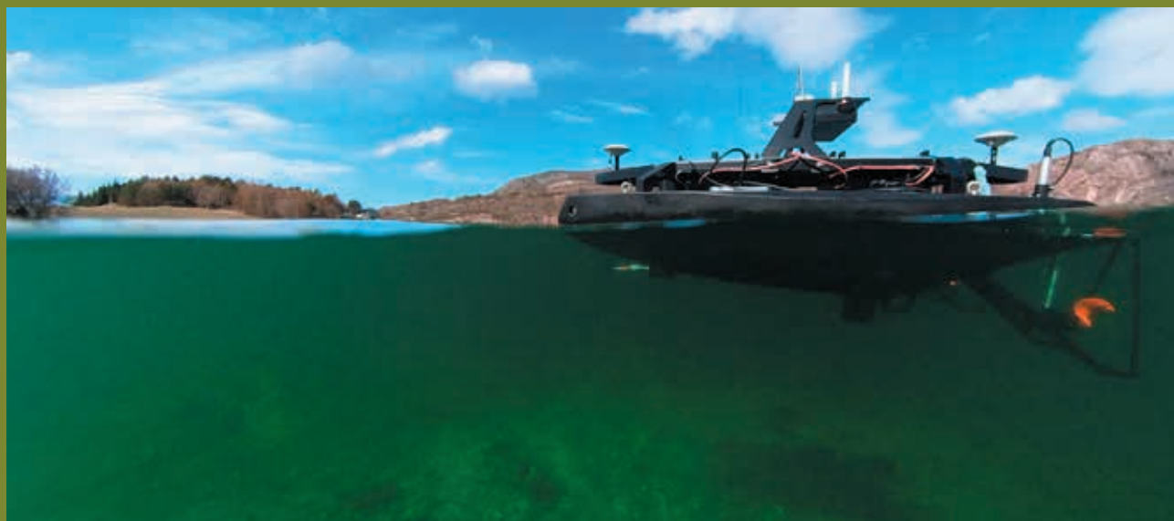
Unmanned surface vehicle with underwater hyperspectral imager for the mapping of shallow habitats. This is part of the NFR- (the Research Council of Norway) funded National Infrastructure Project "SeaBee", for the mapping of shallow habitats along the Norwegian coast with drones.
