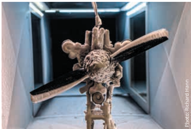
Figure 1: Icing on a propeller during a test campaign in an icing wind tunnel.
