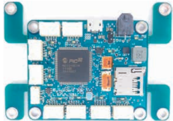
Figure 2: A recent version of the SentiBoard, where various sensors are connected through the various connectors on the top, left and bottom sides; the output goes through the USB connector on the top right, and the functionality is implemented in firmware on the Microchip PIC32 microcontroller.
