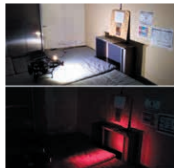
Figure 3: Camera pointed towards target with visible lights (top) or infrared lights (bottom)
