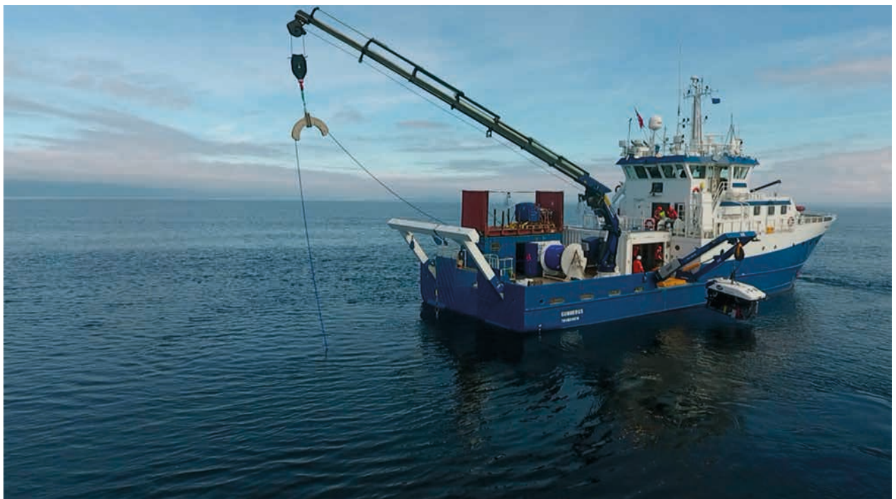
Figure 1: The Subsea Docking Plate being installed using RV Gunnerus in May 2019.
