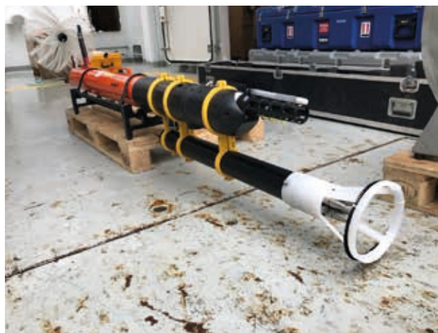
Figure 3: L-AUV Harald with the turbulence sensor mounted.
