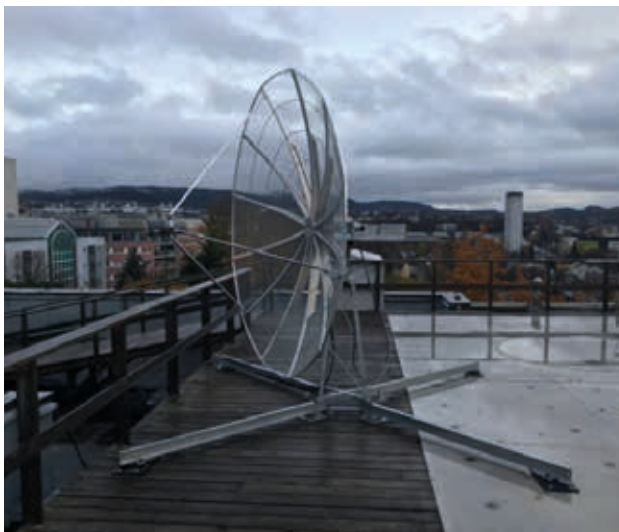
Figure 7: S-band antenna installed at NTNU
