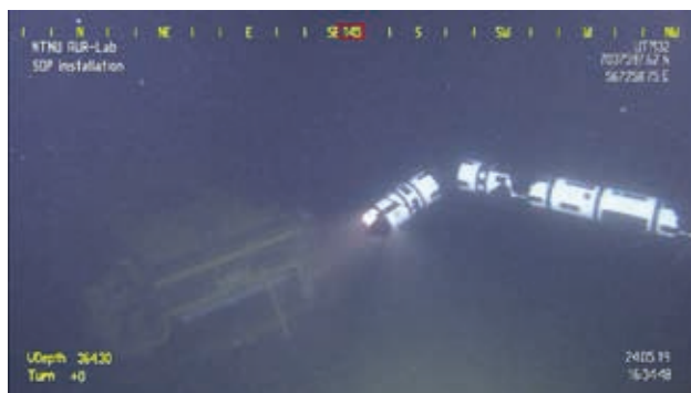
Figure 2: The Eelume underwater vehicle during the testing on the SDP.
