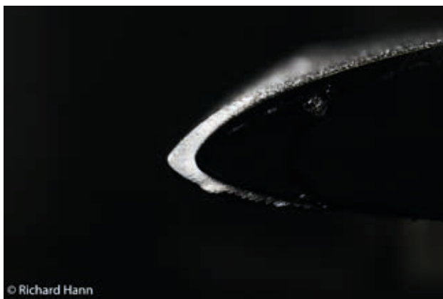
Figure 2: Rime ice on a UAV airfoil in the icing wind tunnel.
