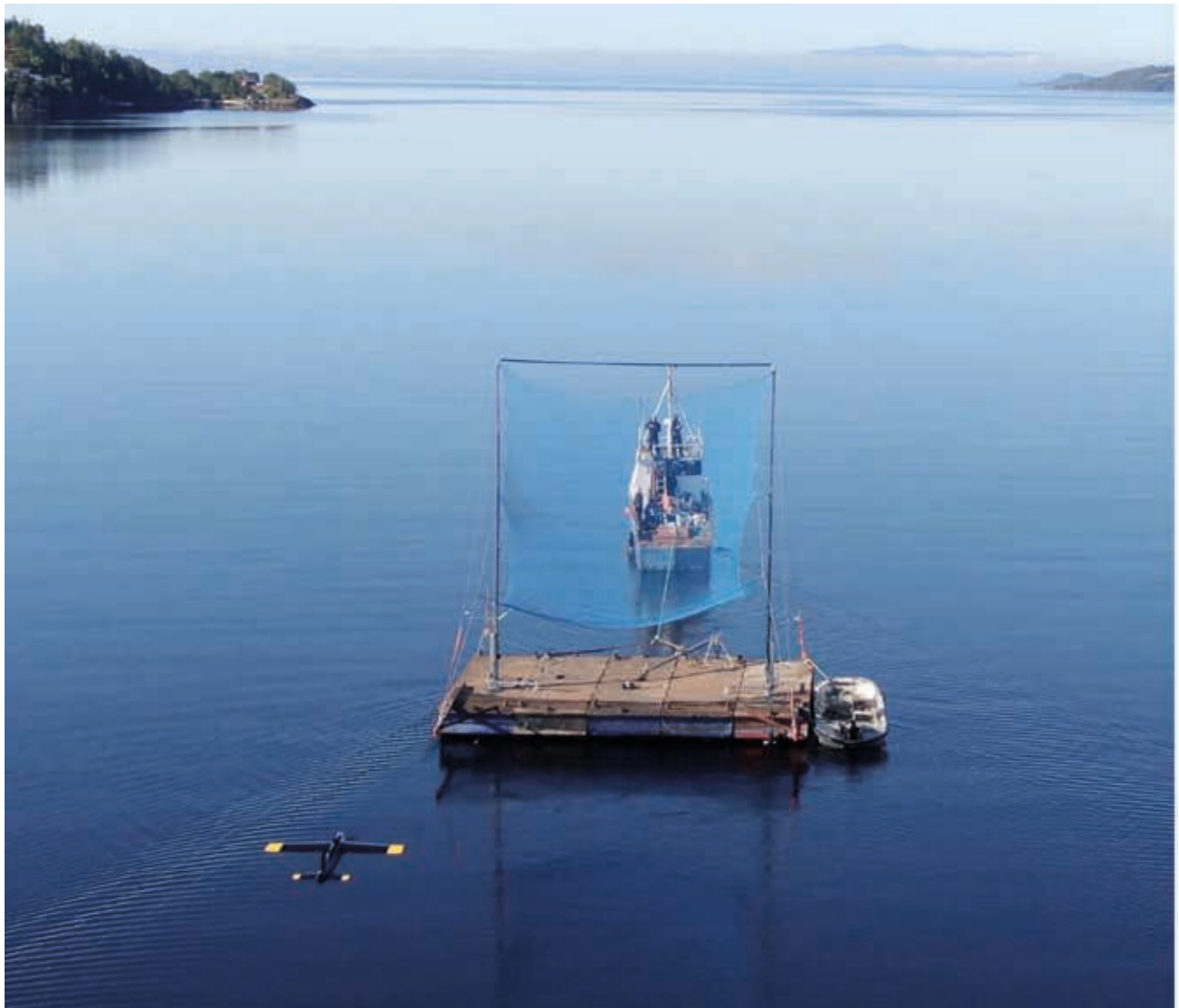
Figure 23: Testing of automatic recovery of fixed-wing UAV in a moving net in Åsenfjorden.
