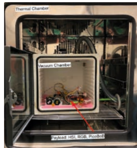
Figure 19: Testing of components in a vacuum chamber inside a thermal chamber
