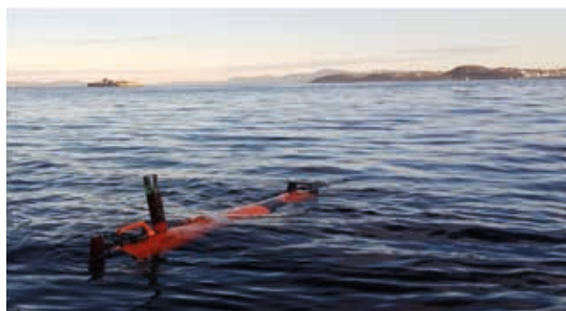
Figure 1: Light Autonomous Underwater Vehicle (LAUV) following phytoplankton hotspots in the coastal waters near Munkholmen in Trondheimsfjorden
