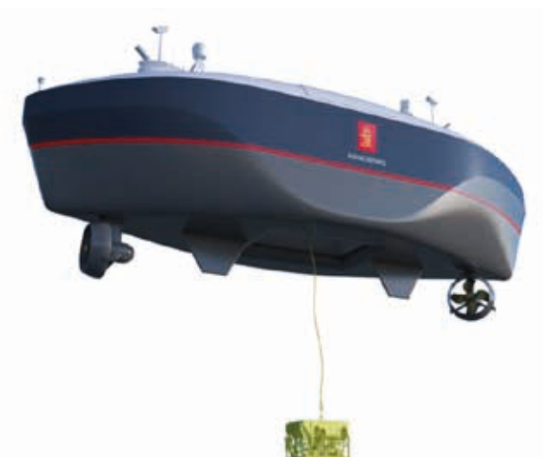
Figure 25: ROV launched and recovered from a relatively small USV. Courtesy Kongsberg Maritime.
