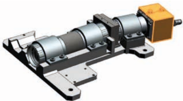
Figure 12: Drawing of custom designed hyper-spectral imager for ocean colour.
