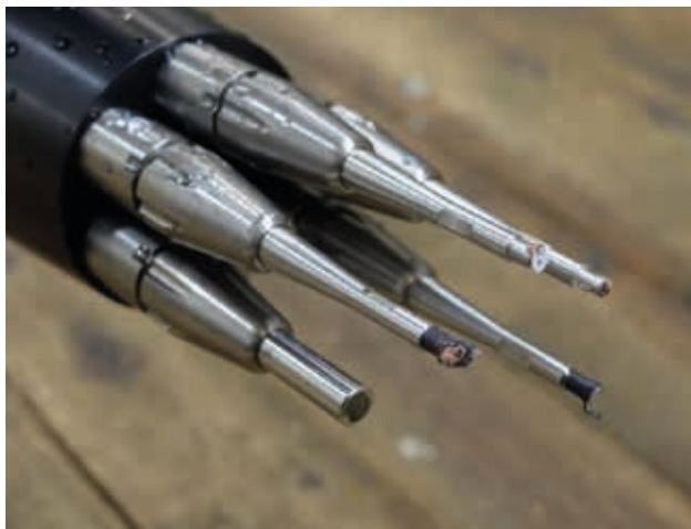
The microstructure probes, broken by the impact with the research vessel. Photo: Ragnheid Skogseth
