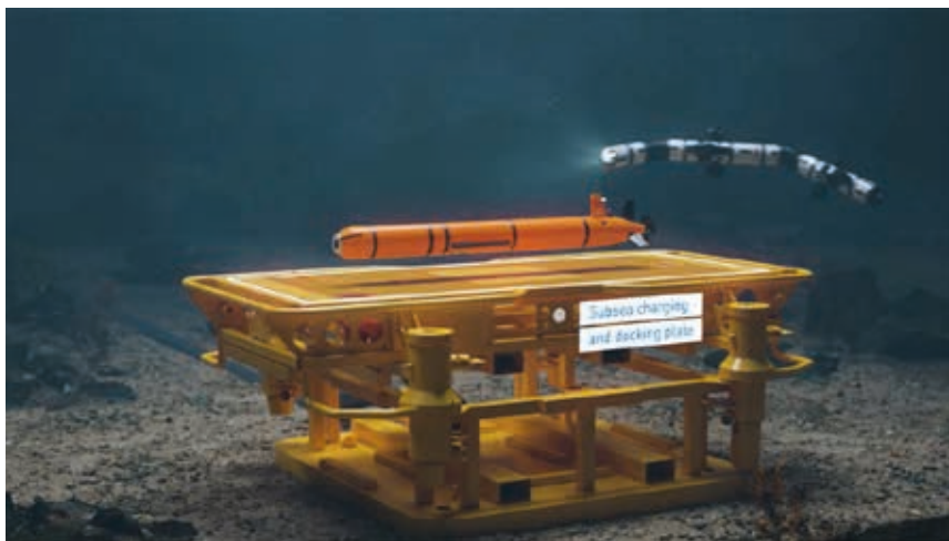
Figure 11: Subsea charging and docking plate in the Trondheimfjord.
