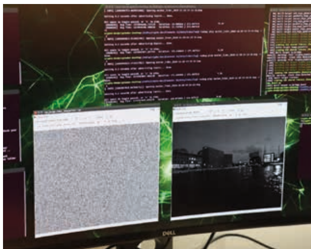
The image on the right is a live feed from an autonomous vessel in the Trondheim Fjord, whereas the image on the left is the same data, but encrypted in order to protect the data.
