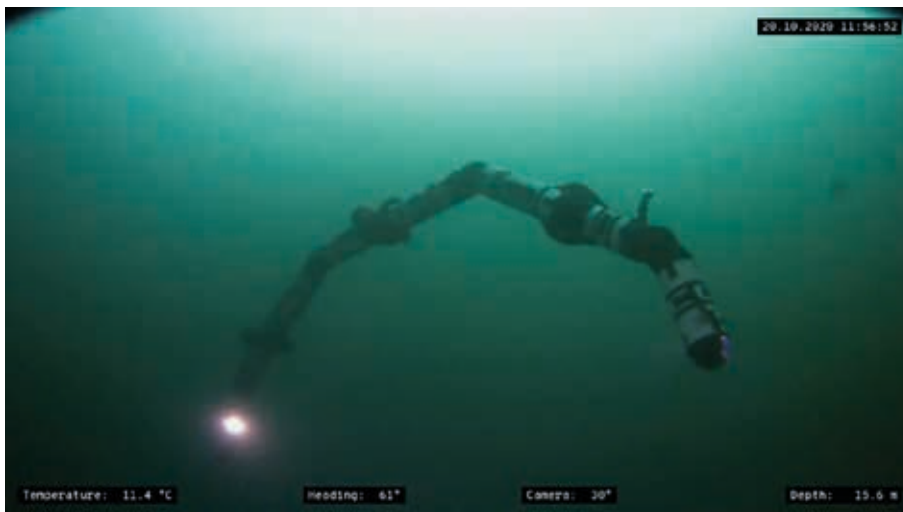
Figure 8: The Eelume underwater vehicle doing a seabed inspection
