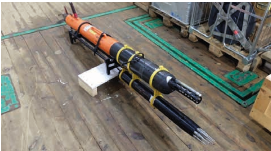
LAUV Harald, carrying the microstructure sensor (AKA the shock absorber). Photo: Ragnheid Skogseth
