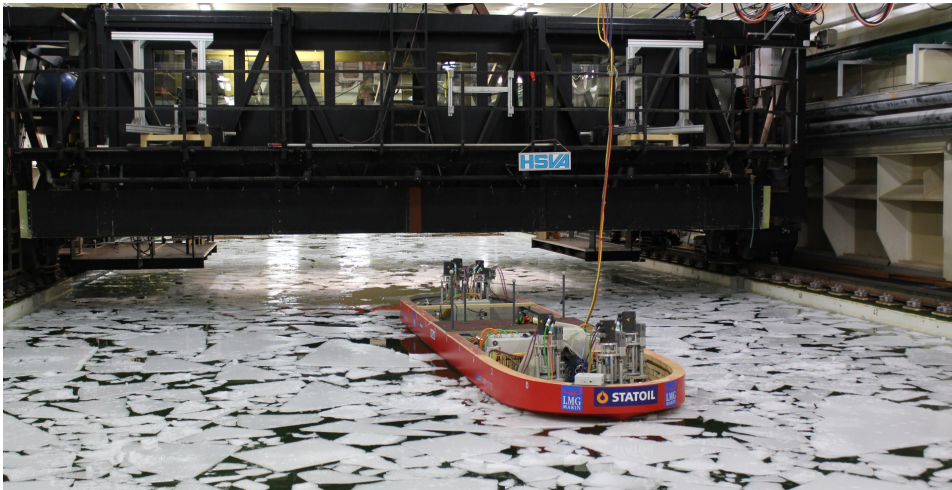
Figure 3.4: Free floating DP experiment at HSVA during the Dynamic Positioning in Ice project. Courtesy of Statoil.
