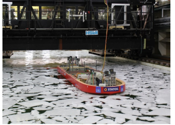
Fig. 7. The model scale Arctic Drillship during experimental testing at HSVA. Courtesy of DYPIC.
