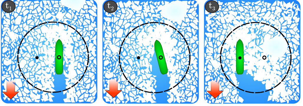
Figure 2. Illustration of manoeuvring to seek the weakest path through the ice, and corresponding utilization of the drifting sea ice for vessel actuation. At t_1 , a potentially significant ice load feature is approaching the vessel, and the position is changed from the hollow circle to the full black circle. At t_2 , the vessel has created an oblique angle while maintaining its upstream position to acquire an actuating starboard ice load. At t_3 , the vessel has utilized the ice load to move into the new position and minimized the oblique angle to minimize the load, allowing the hazardous ice feature to pass.
