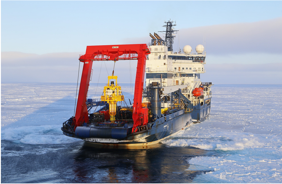
Figure 3.5: Icebreaker Fennica using her azimuth thrusters to clear ice in the North-West Passage 2015. Courtesy of Nordica Master Matti Westerlund and Arctia Ltd.
