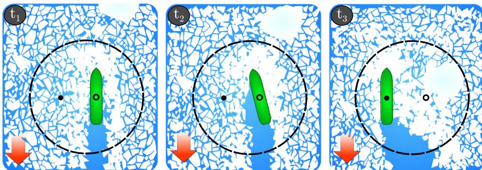
Fig. 13. Illustration of maneuvering to seek the weakest path in the ice and utilization of the drifting sea ice for vessel actuation. At t_1 , a potentially significant ice load feature is approaching the vessel, and the position is changed from the hollow circle to the full black circle. At t_2 , the vessel has created an oblique angle while maintaining its upstream position to acquire an actuating starboard ice load. At t_3 , the vessel has utilized the ice load to move into the new position and minimized the oblique angle to minimize the load, allowing the hazardous ice feature to pass.
