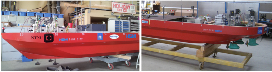
Fig. 2. Hull shape of the Arctic Drill Ship. Left: bow view, right: stern view. White marks indicate the waterline.
