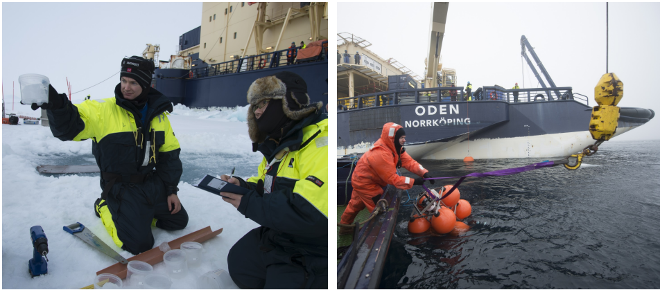
Figure 2.2: Left: Storing ice cores after compression tests. Right: Deploying multi-beam upward looking sonar. Both pictures are from Oden Arctic Technology Cruise 2012. Courtesy Øyvind Hagen and Statoil.
