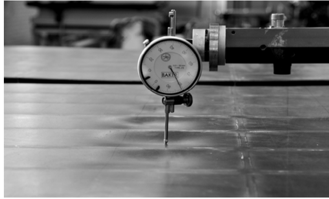
Figure 56: A photograph of the plate damage after Test no. 5.
