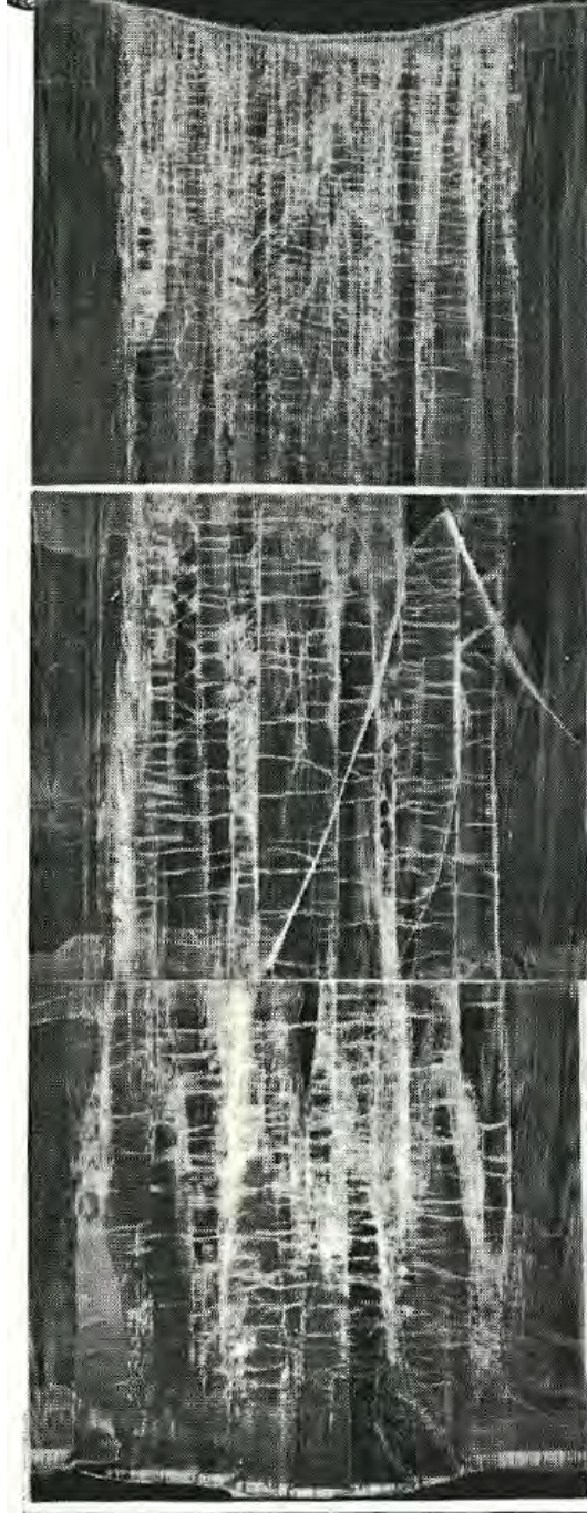
Figure E1: Vertical thin section of ice sample taken with a combination of cross polaroid and reflected light; source: Jones and Sinha (1990).
