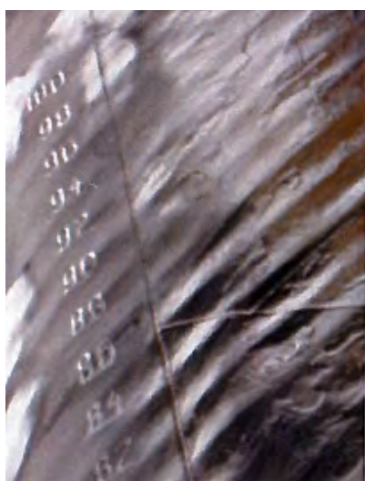
Figure 86: Damage to steel structure caused by ice: permanent deflections of a ship plating caused by ice (from Hänninen (2005)).
