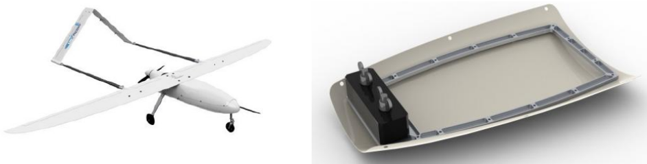
Figure 2.15: The UAV Factory Penguin-B platform (left) and its universal payload mount. The payload is mounted in the front bottom of the Penguin-B UAV.
