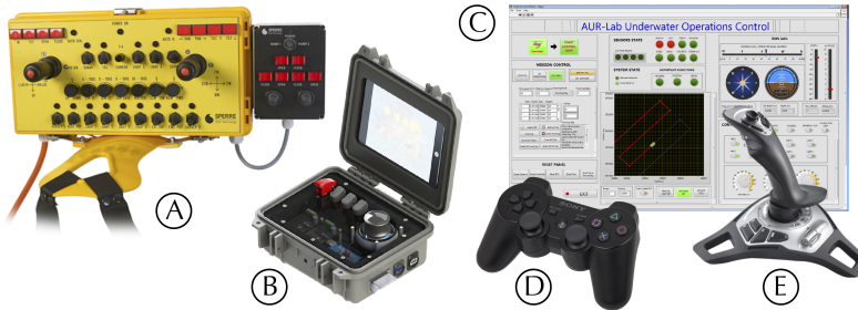
Figure 2.11: Most common ROV control interfaces. (A) shows the combined ROV-manipulator interface that is provided by Sperre AS together with the ROV Minerva and 30k. (B) shows the control panel case used to control small OCROVs (e.g. VideoRay, Saab Seaeye). (C) shows the GUI developed together with the AUR-Lab control system (see Figure 2.3). (D) and (E) show two examples of common off-the-shelf video-gaming joysticks, which are common for fast and low-cost developing and prototyping of DP systems.
