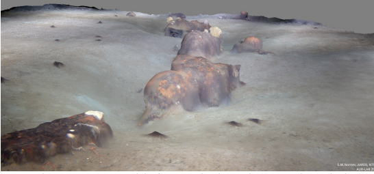
Fig. 6 Photogrammetry model of manmade objects laying on the seabed on the Agdenes dumping field (B in fig 1.). The object in the center of the figure is measured from the photogrammetry model to be 115 cm long and 30 cm in diameter.
