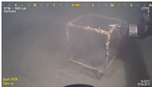
Fig. 10. Here the moment when the box is grabbed is shown: the ROV is kept stable with the HMD and the manipulator is actuated using the joystick depicted in Figure 9.
