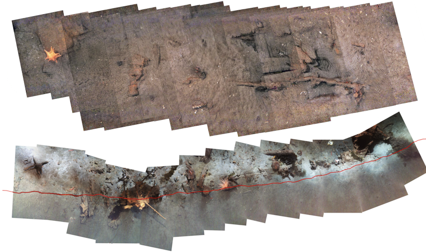
Figure 3.2: Examples of real-time mosaics built while running a transect with the ROV Minerva. The navigation data from the control system has been used to improve the feature matching process and obtain a more correct matching. The ROV usually moves at 0.2 - 0.3 \frac{m}{s} at a constant altitude of 1 - 3m depending by the light conditions and depth. Altitude and speed are mutually selected in order to provide around 30% of overlapping between sequential pictures.
