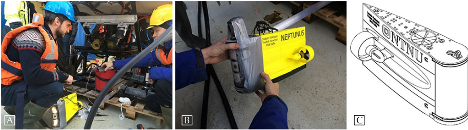
Figure 5.1: Some pictures from the Neptuneus project. (A) Process of integration of the micro-ROV Neptuneus, with the MSROV 30K. (B) The innovative design of the vehicle. (C) A CAD design table.
