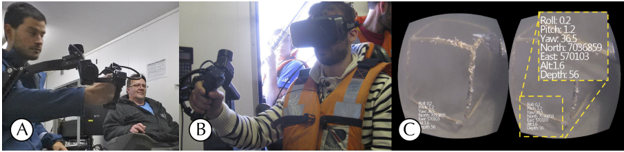
Figure 2.13: Full-scale test of an ROV manipulation work. (A) shows the operation carried from two operators. (B) shows the operator performing the same operation using the HMD. (C) shows the operator's view, which is a stereoscopic video, with an overlay containing the ROV state.
