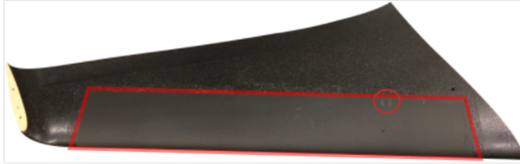
Figure 8.7: X8 Skywalker wing, with thermocouples embedded and applied electro-thermal source. Thermocouple locations are highlighted by a red circle (○) and the electro-thermal source is emphasized by a red square (□).
