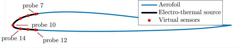
Figure 7.2: Location of virtual sensors on the aerofoil of an X8 Skywalker platform, for a thermodynamic analysis with alternative electro-thermal source layout.
