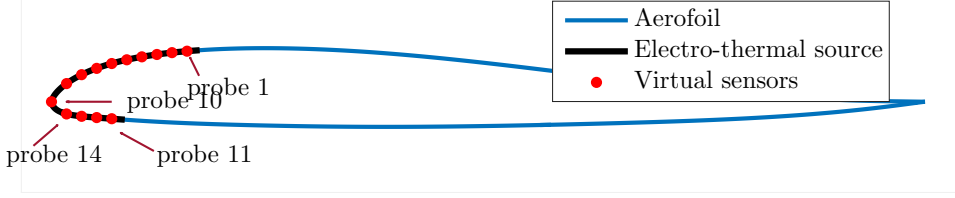
Figure 5.2: Location of virtual sensors on the aerofoil of an X8 Skywalker platform.
