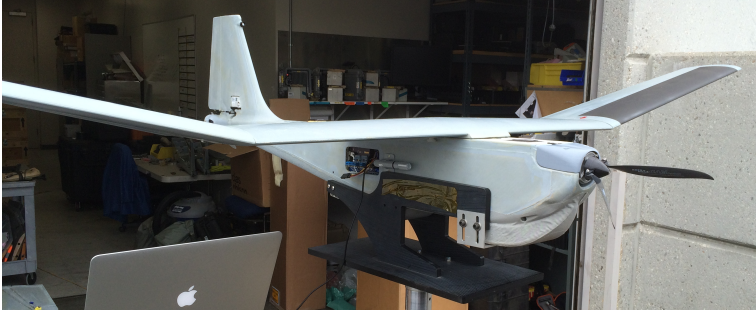
Figure 8.6: Assembled Puma, with IPS retro-fitted.
