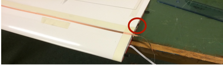
(b) Wing element with wing structure exploited for thermocouple wiring, emphasized by the red circle (○).
