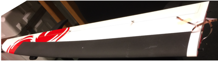
(c) Wing element with electro-thermal source applied to the leading edge.
