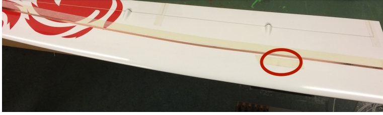
(a) Wing element fitted with copper strips and thermocouples, their location highlighted by the red circle (○).
