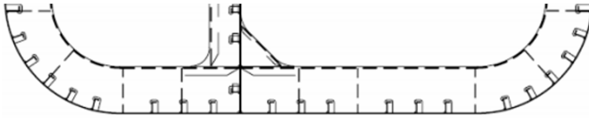
Figure 6.22: Platform column stringer, typical structural layout.
