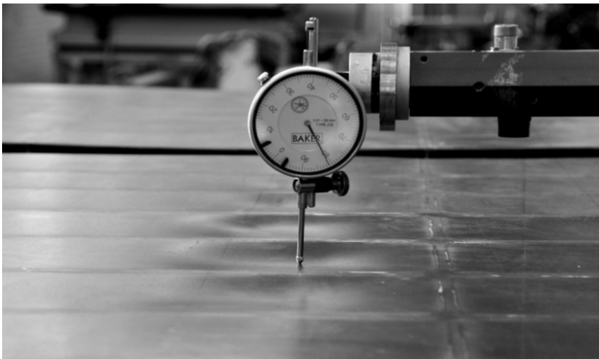
Figure 8.7: Deformation measurement of deformed panel after drop test 2 using a plunger-type gage on a three-axis stand.
