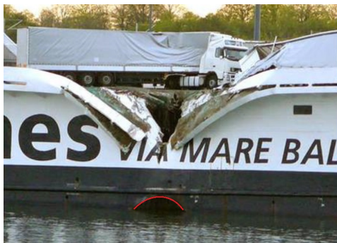
(a) URD. Red line indicates puncture by bulbous bow
