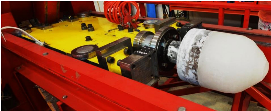
Figure 8.10: Ice sample mounted to the trolley.
