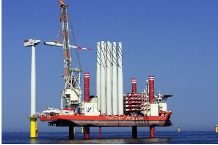
(a) OWT balde installation using a jack-up vessel. Source: https://media.licdn.com/mpr/mpr/shrinknp_800_800/p/6/005/0b7/104/353401b.jpg
