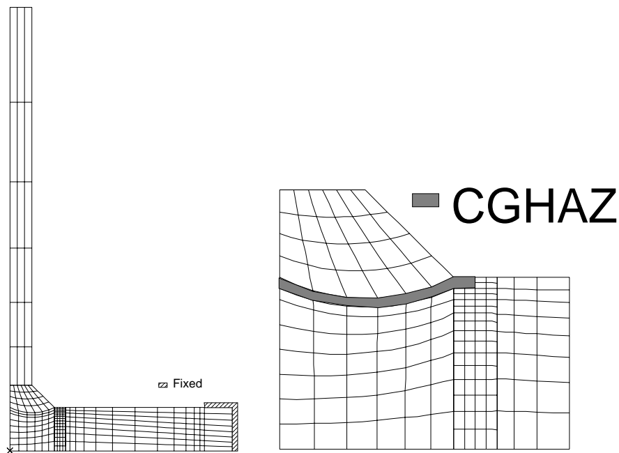
Fig. 7.28 (a) 2D plane strain finite element mesh and boundary conditions at the end of horizontal plate (b) CGHAZ in the finite element model
