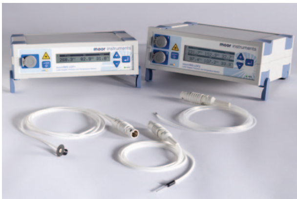
moorVMS-LDF – single and dual channel modules with MemoryChip probes.
