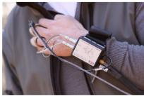
The Portapres® is a true ambulatory blood pressure monitor with a built in memory card (60-hour capacity). Offline BeatScope® software displays patients hemodynamics. Optional real-time and remote solutions are available.
