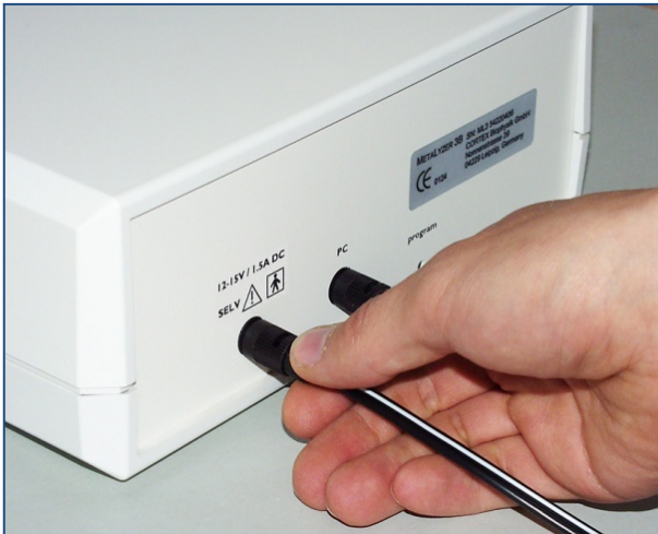
Connecting the power supply cable of the desktop power supply unit to the device
