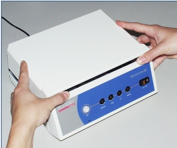
Opening the device housing
