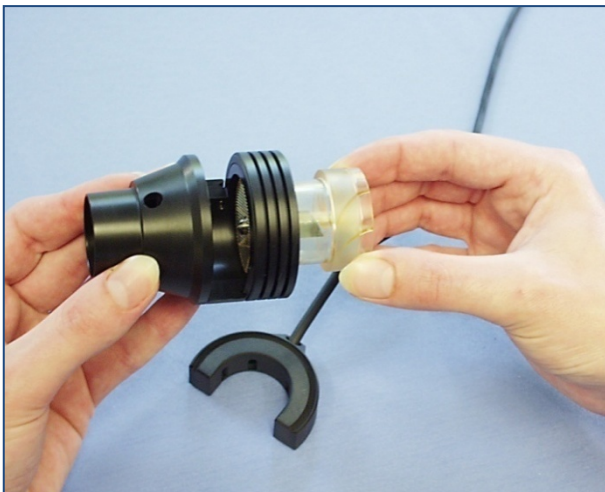
Sliding the turbine out of the housing
