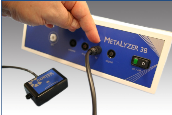
Connecting the POLAR® receiver to the device
