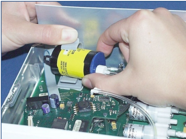
Pulling out the oxygen sensor
