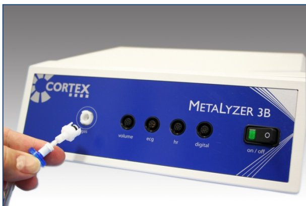
Connecting the sample line to the device
