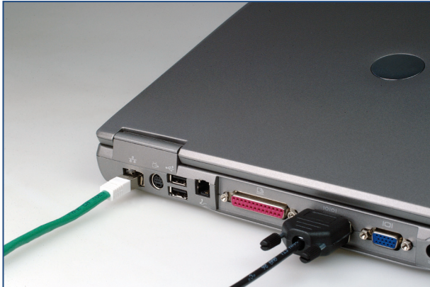
Connecting a workload device cable to a serial port
