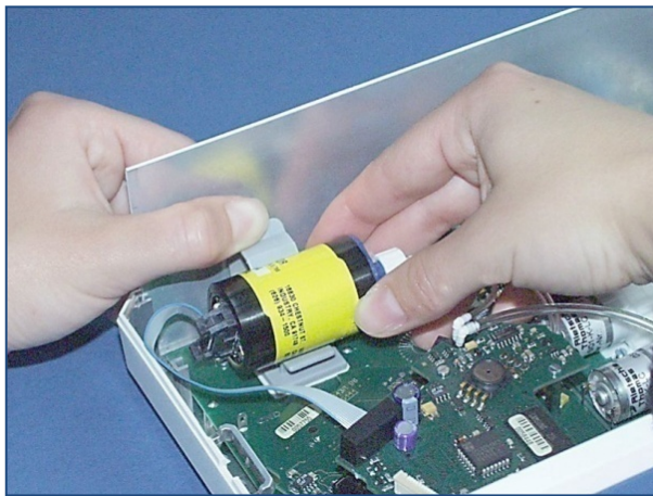
Fastening the oxygen sensor into place
