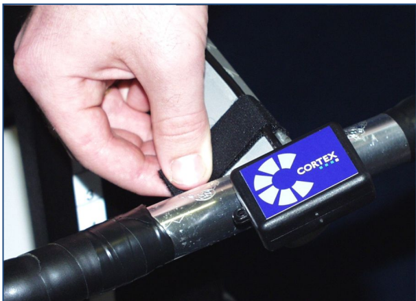
Attaching the POLAR® receiver to the workload device
