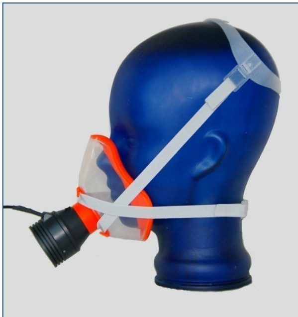
Attaching the volume sensor to the mask
