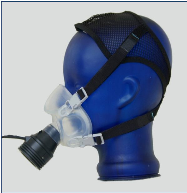
Attaching the volume sensor to the mask
