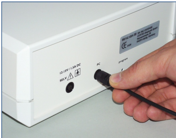
Connecting the PC connection cable to the device
