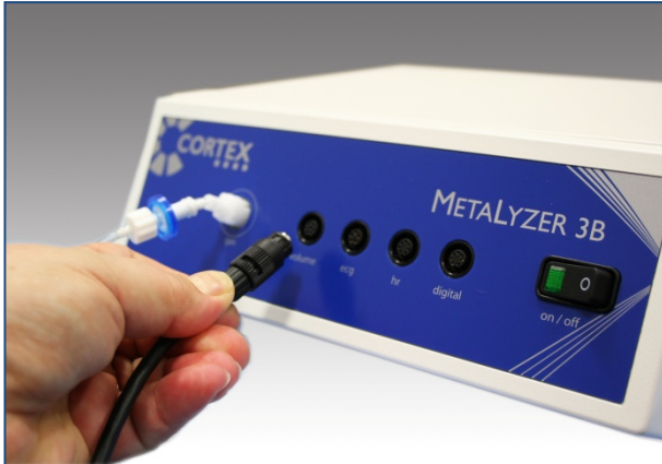
Connecting the volume sensor
