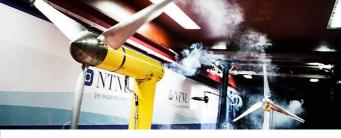
**The Ocean Basin Laboratory** has a depth of 10 metres and a water surface of 50x80m. It is excellent for investing existing or future challenges within marine structures and operations. A total environmental simulation including wind, waves and current offers a unique possibility for testing models in realistic conditions.
