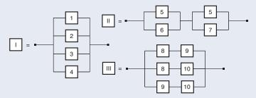
Module II cannot be further partitioned because component 5 is present in both parallel structures.
