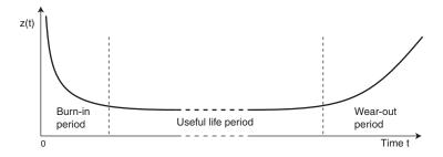
Mechanical components are often assumed to have a failure rate function with a bathtub shape.
