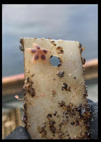
Conditioning film  $\rightarrow$  Adherent Bacteria  $\rightarrow$  Bacterial Biofilm  $\rightarrow$  Microalgae and Diatoms  $\rightarrow$  Larva of Invertebrates and Invertebrates
