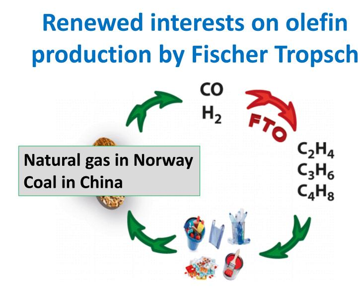
Possible to produce olefin via synthesis gas from natural gas, coal and biomass
