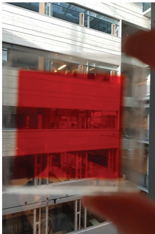
Transparent solar cells could be used as part of a building's window or facade. Photo: David Moe Almenningen
