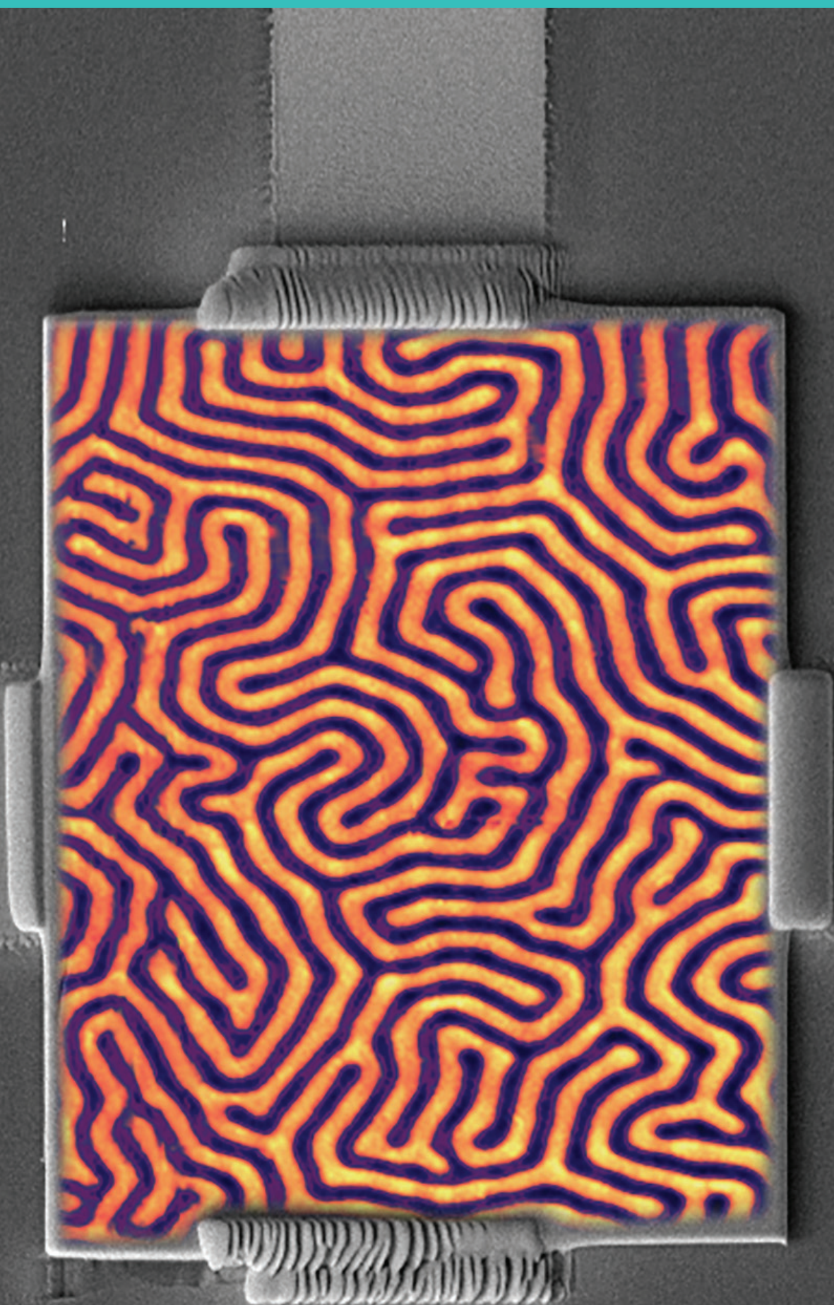
Magnetic lamella in a 300 nm thin film of Fe 3 Sn 2 . Photo: Erik Dobloug / NTNU NanoLab.
