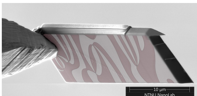
First steps in the preparation of a domain wall device. Photo Erik Roede/NTNU NanoLab
