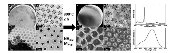
SEM images of diatom frustules before and after reaction along with corresponding observed Raman shift and luminescence.
